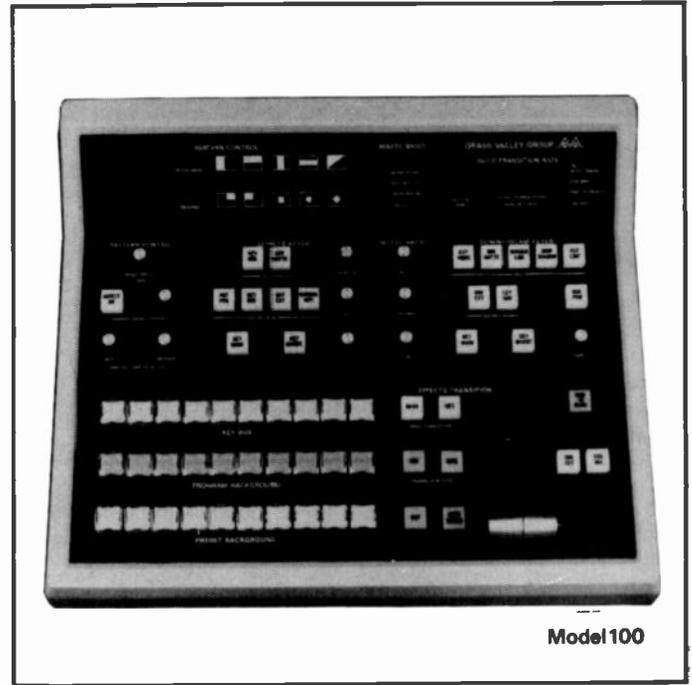
The 100CV features non-looping video inputs, 8 in all, and 3 sets of BNC connectors for every input. Utilizing the same control panel as the 100 Production Switchers, the 100CV Component Video Production Switcher has updated electronics that incorporates as standard equipment many of the features offered as options on the 100.
