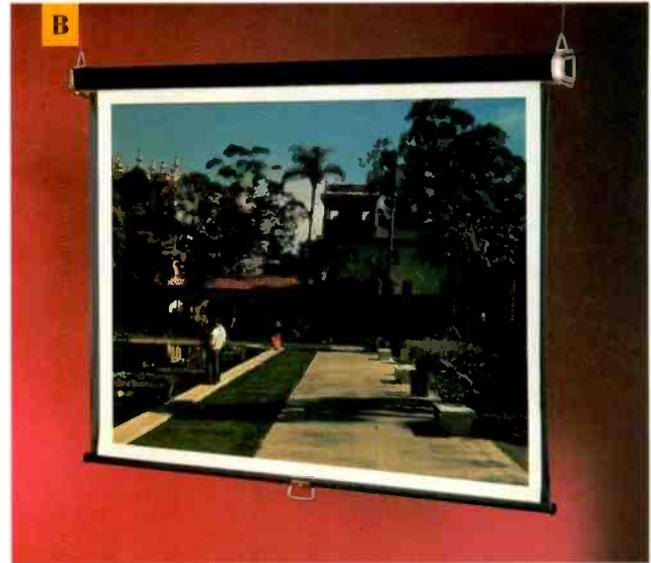
**To Calculate the Screen Size:** Determine the distance between the screen and the last row of the audience. Divide that distance by 6 for screen width of 4x3 ratio projected images, or divide the distance by 8 for screen width of square projected images.
