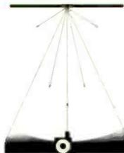
**Glass Beaded** screens give a fantastic brilliance in the viewing angle cone. Most of the projected light is reflected back to the audience. Especially suitable for projectors with poor light output and for use in long, narrow rooms.
