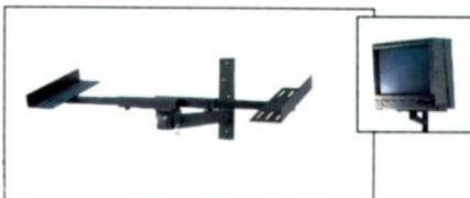
**LTM-1** is a wall mount. It will accommodate most 19" to 27" TV receivers. Adjusts from 16" to 30" width. TV rests on 3" wide 1/8" steel supports which are slotted. Super bond adhesive strips and safety strap included. TV bolts, bonds and straps to mount. Maximum forward tilt 10° and 180° swivel capability. Mount to wood, brick or concrete surfaces. Installations vary; therefore, mounting hardware is not included. Ships in 1 carton. Weight 17 lbs. . . . **\$150**
