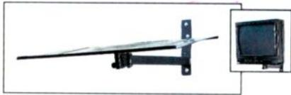
**LTE-1** is a platform wall mount. It will accommodate most 19" and 20" TV receivers. TV rests on 20" wide by 13½" deep heavy-gauge steel platform with ½" front retainer lip. Safety strap included. Maximum forward tilt 15° and 240° swivel capability. Installations vary; therefore, mounting hardware is not included. Load capacity 90 lbs. Wt. 18 lbs. . . . . **\$99**
