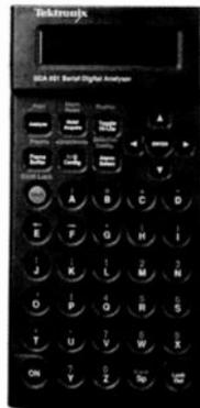
**Video Format Analysis** Detects and reports on signal parameters including line/field rate, clock rate, active picture resolution (8- or 10-bit) and embedded audio status.
