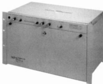
The DJ-4101 mainframe provides 14 module mounting spaces, DC power and a lockable security cover for the System 41° signal processing modules. The system operator control panel includes a power on/off switch and LED indicator for DC bus power. A monitor provides an input selection switch, a 10-segment LED peak level display and a 3W amplifier. 2 balanced attenuators, useful for system level control, are also supplied.
