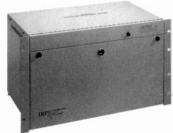
The DJ-4100 mainframe provides 14 module mounting spaces, DC power and a lockable security cover for the System 41° signal processing modules. The system operator is furnished with a power on/off switch and a power/on LED which monitors both the positive and negative DC output power to the mainframe modules.
