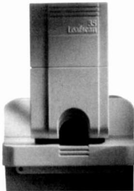
acquire plug-in module. Intel 80188 internal command processor. Motorola 56000 DSP for data correction and averaging. Macintosh (24-bit color systems, 8M byte RAM) host compatibility. GPIB or SCSI2, switch selectable ID switch for daisy-chaining SCSI2 host interfaces. Both scanners support Leaf 16-bit file formats.
