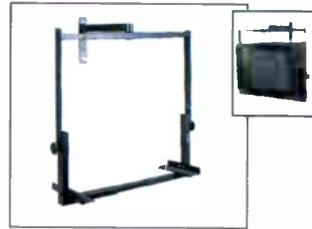
**LTE-5** is an adjustable yolk-style wall mount. It will accommodate most 19" to 27" TV rece. Adjust from 21½" to 33" without LTEV accessory VCR shelf, or 23½" to 33" with LTEV. Heavy-gauge tubular steel construction with 3" wide by 10" long steel supporters, covered in nc material. Heavy-duty 2" wide safety strap included. Maximum forward tilt 15° and 24° capability. Installations vary; therefore, mounting hardware is not included. Load capacity 1 Wt. 25 lbs. . . . .
