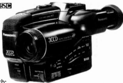
iris/white balance • 5-pin edit terminal • Digital auto focus • f/1.4 • Focal length 5-40mm • Auto iris • Filter diameter 49mm • Mic in • Audio/video outputs • Approximately 5.7 lbs.
