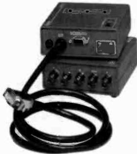
The RGB 109 Plus is designed to provide high resolution performance for the anticipated yet to be announced high scan 48 to 90kHz graphics modes of Super VGA. A separate buffered workstation monitor output is the highest resolution method of interfacing for maintaining the original signal bandwidth. No input cable purchase required.
