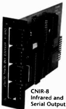
CNIR-8 Infrared and Serial Output
