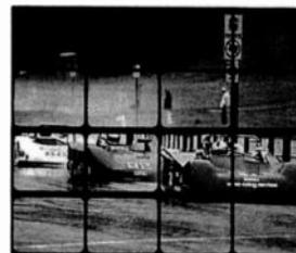
1 x 4—The IVW-400 expands the image to 16X actual size. This mode is designed for use with horizontally oriented video. A horizontal key window of 1 quarter the expanded image is displayed by each processor, while scroll capability allows for alignment.
