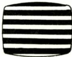
FIG. 3. HORIZONTAL BARS PRODUCED BY 400CPS MODULATION ON SCREEN OF TV RECEIVER
