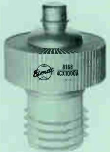
This high-power ceramic-metal tetrode is an excellent choice for applications where class-AB<sub>1</sub> operation is desired. It is capable of delivering more than 1500 watts plate output power per tube in audio or r-f service without requiring grid driving power. It is recommended for use in new equipments.
