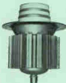
Recommended for use as a modulator, oscillator or amplifier, the 4CV35,000A is usable to 110 megacycles. With a plate voltage of 10 kV in Class-C service, the tube is capable of over 35 kilowatts output power. The plate dissipation of 35 kilowatts allows use of the 4CV35,000A in low efficiency Class-AB<sub>1</sub> circuits.
