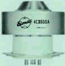
The Eimac 4CX600A is a new ceramic-metal tetrode with low lead inductances and low interelectrode capacitances and is designed especially for distributed amplifier and UHF service.
