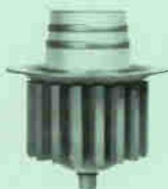
A vapor-cooled version of the popular 4CX5000A, the 4CV20,000A has a plate dissipation rating of 20 kilowatts. Two of these tubes in a push-pull, Class-AB<sub>1</sub> amplifier will produce 35 kilowatts output.
