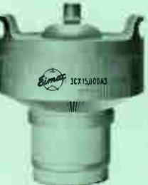
A new addition to Eimac's line of ceramic-metal triodes, the 3CX15,000A3 is a medium-mu triode designed especially for rf heating service. Six amperes of dc plate current is available from a one kilowatt filament and the grid structure is rated at 500 watts. Adequate forced-air cooling permits 15 kilowatts of plate dissipation. The 3CX15,000A3 is also useful as a linear or plate-modulated rf amplifier.
