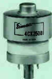
A 250-watt general purpose external-anode tetrode featuring ceramic-metal construction. This compact power tube can be used at maximum ratings at frequencies up to 500 megacycles. It is recommended for use in equipments of new design. The 4CX250F is identical in all respects except for a heater rated at 26.5 volts.
