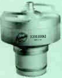
Here is a new ceramic-metal medium-mu triode designed for industrial-heating oscillator service. It features a large thoriated-tungsten filament with ample reserve emission and an integral anode cooler with the inherent ability to withstand large overloads. It is intended for use through 140 megacycles, also as a grounded-grid FM amplifier developing 20 kilowatts useful output power.
