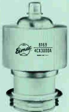
The 4CX3000A is a new ceramic-metal tetrode designed especially for class-AB<sub>1</sub> linear amplifier service. In such service, the intermodulation distortion products produced by the 4CX3000A are of very low level, typically 32 to 44 db below PEP level, depending on operating conditions. The ample grid and screen dissipation ratings also make the 4CX3000A attractive for use as a class-C amplifier. The 4CX3000A is first choice for modern, new equipment design.
