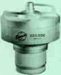
The new Eimac 3CX10,000A7 is a ceramic-metal zero-bias triode intended for use in grounded-grid linear amplifiers delivering 20 kilowatts of useful output power. Because of its low intermodulation distortion characteristics the 3CX10,000A7 is particularly well suited for single-sideband amplifiers. Two tubes operating in a push-pull audio amplifier under class-B zero-bias conditions will deliver up to 45 kilowatts of useful output power.
