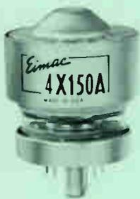
The veteran of external-anode tetrodes, and an Eimac original, continues to enjoy its deserved popularity. Recent tube improvements have made possible increases in maximum plate voltage and plate-dissipation ratings. In Class-AB or Class-C service an input power of 500 watts is now allowed at frequencies up to 150 megacycles. The 4X150D is a 26.5 volt heater version of the 4X150A.
