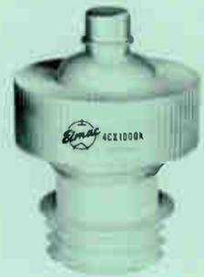
This high-power ceramic-metal tetrode is electrically identical to the 4CX1000A, but gives improved performance at UHF due to its soliding screen terminal. This terminal surface improves isolation between input and output circuits to a marked degree and insures stable UHF operation as a class-AB<sub>1</sub> amplifier.
