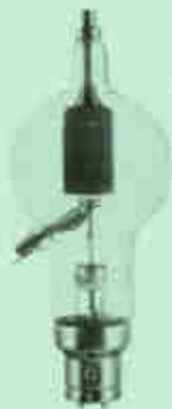
The 450TH is a high-power general-purpose triode with a 450-watt plate-dissipation rating and is cooled by radiation and convection. It has an amplification factor of 38; it is useable at maximum ratings through 40 megacycles.
