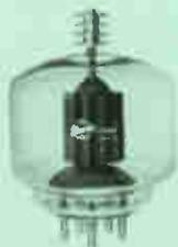
The Eimac 3-400Z is a new zero-bias triode intended for linear amplifier applications. This tube may be used as a Class B R-F amplifier in either the grid-driven or cathode-driven connection, or two 3-400Z's may be used in push-pull as a grid-driven Class B audio amplifier or modulator. At a plate voltage of 3000 volts 1KW PEP input can be run with a single 3-400Z, providing a power gain of over 20 in the cathode-driven connection.
