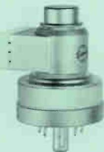
Eimac's new quick-heat tetrode, featuring a 100 millisecond warm-up with "hot-shot" filament voltage or a one second warm-up at normal filament voltage. The 4CS100L is equipped with a beryllium oxide ceramic brazed to the anode. The excellent thermal conductivity of BeO combined with its electrical insulating properties permits flexibility in heat-sink cooling of this tube.
