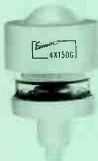
One of the forerunners in external-anode coaxial-based tetrodes, the 4X150G continues to deliver long life and high reliability in VHF and UHF applications. It is intended for use in CW service at frequencies up to 1200 megacycles and is useful in pulse service at frequencies up to 1500 megacycles.
