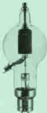
The 450TL is a high-power general-purpose triode with a 450-watt plate-dissipation rating and is cooled by radiation and convection. It has an amplification factor of 18; it is useable at maximum ratings through 40 megacycles.
