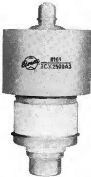
This popular high-power triode is widely employed in AM, FM, and TV service. Its coaxial filament and grid terminals insure low-inductance connection to these electrodes and allow operation at maximum ratings through 75 MHz. The use of an external forced-air-cooled anode results in a compact structure with high power-handling capability.
