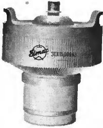
The 3CX15,000A3 is a medium- $\mu$  triode designed especially for rf heating service. Six amperes of dc plate current is available from a one kilowatt filament and the grid structure is rated at 500 watts. Adequate forced-air cooling permits 15 kilowatts of plate dissipation. The 3CX15,000A3 is also useful as a linear or plate-modulated rf amplifier.
