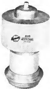
Eimac's largest, forced-air cooled power tetrode has a plate dissipation rating of 35 kilowatts and is usable to 20,000 plate volts in Class-C and Class-AB amplifier service. A single 4CX35,000C will deliver over 100 kilowatts of CW power as a Class-C power amplifier or oscillator.
