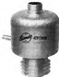
The 4CV1500B is a ceramic-metal, vapor and forced air cooled radial beam tetrode with a rated maximum plate dissipation of 1500 watts. It is a low-voltage, high-current tube specifically designed for exceptionally low intermodulation distortion and low grid interception. The low distortion characteristics make the 4CV1500B especially suitable for RF and AF linear amplifier service.
