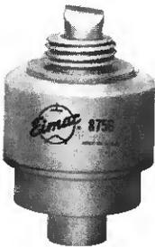
The 8756 is a miniature frequency-stable planar triode for pulse applications up to 2500 MHz at full ratings. The tube is designed for high pulse current operation.
