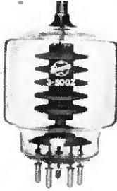
The 3-500Z is a compact power triode intended for use as a zero-bias Class B amplifier in audio or radio-frequency applications. Operation with zero grid bias simplifies associated circuitry by eliminating the bias supply. In addition, grounded-grid operation is attractive because a power gain as high as twenty times can be obtained with the 3-500Z in a cathode-driven circuit.
