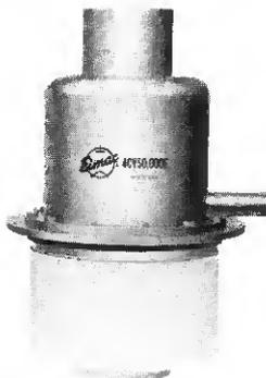
The 4CV50,000E is a ceramic-metal, vapor-cooled tetrode intended for use at the 50 to 100 kW output power level. It is recommended for use as a Class C RF amplifier or oscillator, a Class AB RF linear amplifier or a Class AB push-pull AF amplifier or modulator. The 4CV50,000E can also be used as a plate and screen modulated Class C RF amplifier.
