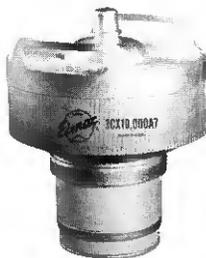
The Eimac 3CX10,000A7 is a ceramic-metal zero-bias triode intended for use in grounded-grid linear amplifiers delivering 20 kilowatts of useful output power. Because of its low intermodulation distortion characteristics the 3CX10,000A7 is particularly well suited for single-sideband amplifiers. Two tubes operating in a push-pull audio amplifier under class B zero-bias conditions will deliver up to 45 kilowatts of useful output power.
