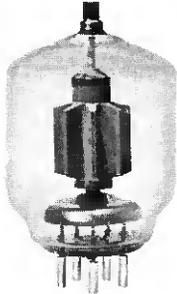
A new medium-mu triode, the 5867A is capable of over one kilowatt input to 100 Mc. It is useful as a Class AB amplifier, Class C amplifier or industrial oscillator. The plate dissipation rating is 375 watts.
