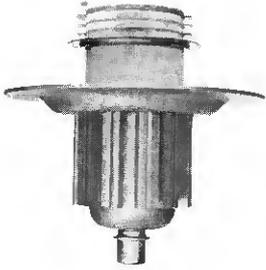
This vapor-cooled version of Eimac's 4CX3000A offers a conservative plate dissipation rating of 8000 watts. It is recommended for Class-AB audio and radio-frequency applications as well as Class-C rf amplifier service.
