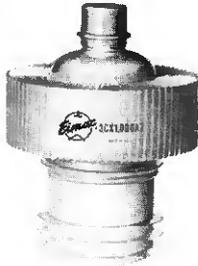
The 3CX1000A7 zero-bias triode features ceramic-metal construction and a mesh thoriated-tungsten filament. Positive socketing is provided by three breechblock terminal surfaces. This tube is intended for class-B linear amplifier service in either the grid-driven or cathode-driven connection. It is equally attractive for use at audio frequencies or at radio frequencies through the TV broadcast bands. It is recommended for use in new equipment.
