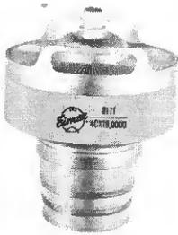
This Eimac tetrode is electrically identical to the 4CX5000A except for its plate dissipation rating and is intended for use where the extra plate dissipation is a necessity. It may be used at maximum ratings through 30 MHz and at slightly reduced ratings through the FM broadcast band.
