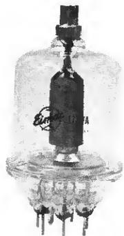
The 177WA beam pentode is a ruggedized version of the 177A with which it is directly interchangeable. The 177WA may be mounted in any position and will withstand high levels of shock and vibration. The tube incorporates a unique vane-type suppressor grid which permits high power output at relatively low plate voltages and provides excellent characteristics for use as a linear RF or audio amplifier.
