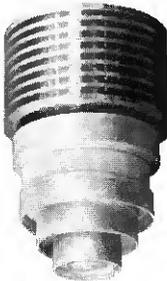
The 6816 is a small coaxial power tetrode designed for UHF power amplifier and oscillator service up to 1200 MHz. Coaxial construction makes this tube suitable for cavity circuits.
