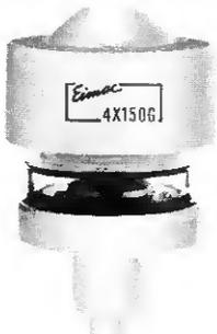
One of the forerunners in external-anode coaxial-based tetrodes, the 4X150G continues to deliver long life and high reliability in VHF and UHF applications. It is intended for use in CW service at frequencies up to 1200 MHz and is useful in pulse service at frequencies up to 1500 MHz.
