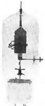
The 254W is a radiation-cooled tube suitable for use as an RF power amplifier, frequency multiplier or oscillator, and as an AF power amplifier and modulator. The tube is widely used in base-station communications equipment and is exceptionally efficient in VHF operation.
