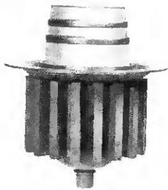
A vapor-cooled version of the popular 4CX5000A, the 4CV20,000A has a plate dissipation rating of 20 kilowatts. Two of these tubes in a push-pull, Class-AB<sub>1</sub> amplifier will produce 35 kilowatts output.
