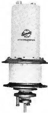
The 4CW250,000A and 4CW250,000V are identical ceramic-metal, water-cooled power tetrodes except that the 4CW250,000V contains an integral ion vacuum pump which may be used to check the tube's vacuum condition during storage or to restore the vacuum of a tube which has been damaged by overheating in service. The tubes are intended for use in the 250 to 500 kW output power range.
