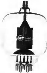
The Eimac 3-1000Z is a zero-bias triode intended for linear amplifier applications. This tube may be used as a class-B R-F amplifier in either the grid-driven or cathode-driven connection, or two 3-1000Z's may be used in push-pull as a grid-driven class-B audio amplifier or modulator. At a plate voltage of 3000 volts, 2KW PEP input can be run with a single 3-1000Z, providing a power gain of over 20 in the cathode-driven connection.
