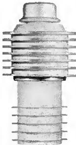
The 4CX125C is a horizontally-finned version of the 4CX300A and is intended for use where transverse air cooling is desired. It is also useful where anode power is dissipated by liquid immersion. Its electrical characteristics are identical to those of the 4CX300A with the exception of plate dissipation which is established at 125 watts with air cooling. It is ideally suited for applications where shock and/or vibration are experienced. The 4CX125F is an identical tube with a 26.5 volt heater.
