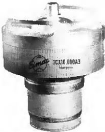
Here is a ceramic-metal medium-mu triode designed for industrial-heating oscillator service. It features a large thoriated-tungsten filament with ample reserve emission and an integral anode cooler with the inherent ability to withstand large overloads. It is intended for use through 140 MHz, also as a grounded-grid FM amplifier developing 20 kilowatts useful output power.
