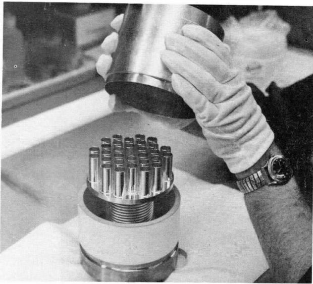
**Final Assembly of VacCap\* Variable Vacuum Capacitor**
