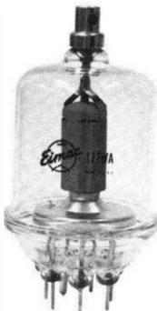
The 177WA beam pentode is a ruggedized version of the 177A with which it is directly interchangeable. The 177WA may be mounted in any position and will withstand high levels of shock and vibration. The tube incorporates a unique vane-type suppressor grid which permits high power output at relatively low plate voltages and provides excellent characteristics for use as a linear RF or audio amplifier.
