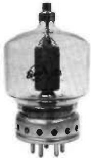
The 6569 is a high-mu power triode designed especially for grounded-grid RF amplifier service, but is also capable of good performance in other applications. Because of its high amplification factor and high perveance, the 6569 will give power gains as high as ten in grounded-grid amplifier applications. Because of internal shielding, neutralization is not required.
