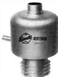
The 4CV1500B is a ceramic-metal, vapor and forced air cooled radial beam tetrode with a rated maximum plate dissipation of 1500 watts. It is a low-voltage, high-current tube specifically designed for exceptionally low intermodulation distortion and low grid interception. The low distortion characteristics make the 4CV1500B especially suitable for RF and AF linear amplifier service.
