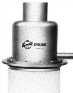
The 4CV50,000E is a ceramic-metal, vapor-cooled tetrode intended for use at the 50 to 100 kW output power level. It is recommended for use as a Class C RF amplifier or oscillator, a Class AB RF linear amplifier or a Class AB push-pull AF amplifier or modulator. The 4CV50,000E can also be used as a plate and screen modulated Class C RF amplifier.
