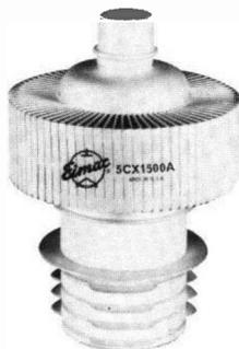
The 5CX1500A is a ceramic-metal power pentode designed to be used as a Class AB<sub>1</sub> linear amplifier in audio or radio-frequency applications. Its low intermodulation distortion characteristics make it especially suitable for single-sideband service.
