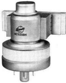
The 4CS250H and 4CS250HA are conduction-cooled tetrodes having the basic electrical characteristics of the 4CX350A. These tubes are intended primarily for class AB<sub>1</sub> linear service. They have high trans-conductance and produce full output with extremely low drive power.
