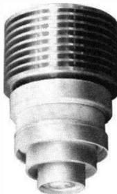
The 6884 is a small coaxial tetrode designed for UHF power amplifier and oscillator service up to 1200 MHz. The coaxial construction makes this tube suitable for cavity circuits. This tube is identical to the 6816 except for heater voltage.
