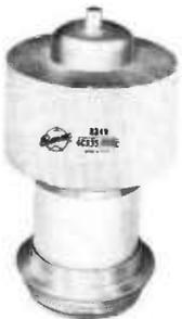
Eimac's largest, forced-air cooled power tetrode has a plate dissipation rating of 35 kilowatts and is usable to 20,000 plate volts in Class-C and Class-AB amplifier service.
