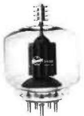
The Eimac 3-400Z is a new zero-bias triode intended for linear amplifier applications. This tube may be used as a Class B R-F amplifier in either the grid-driven or cathode-driven connection, or two 3-400Z's may be used in push-pull as a grid-driven Class B audio amplifier or modulator. At a plate voltage of 3000 volts 1KW PEP input can be run with a single 3-400Z, providing a power gain of over 20 in the cathode-driven connection.
