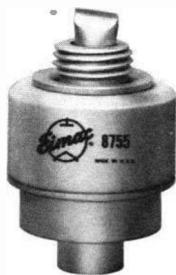
The 8755 is a miniature, frequency-stable planar triode for advanced airborne and space applications up to 3000 MHz at full ratings. The rugged ceramic-metal pulse tube is designed for high-voltage, high-pulse current operation and features large contact areas for improved electrical paths. The tube may be used as an amplifier or an oscillator and employs an arc-resistant cathode.
