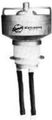
The 3CX10,000H3 is an air-cooled ceramic-metal power triode designed primarily for use in industrial radio-frequency heating service. Its air-cooled anode is conservatively rated at 10,000 watts of plate dissipation. Input of 40,000 watts is permissible up to 90 MHz. Plentiful reserve emission is available from its 750 watt filament. The grid structure is rated at 250 watts.
