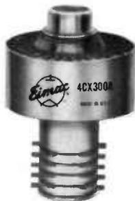
This rugged ceramic-metal tetrode with unique breechblock basing has electrical characteristics similar to other tubes in the 4X150 and 4X250 families but is especially suited for service in severe environments. Its unusual internal construction assures reliable operation at acceleration levels up to 20 g's. Suitable for service from dc to 500 MHz, the 4CX300A is first choice for use in new equipment where shock and/or vibration are expected.
