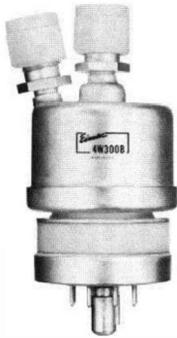
A general-purpose radial-beam tetrode with electrical characteristics similar to those of the Eimac 4X250B, this water-cooled version is intended for use where reserve anode dissipation is desired or where the use of water is a convenience. Maximum ratings apply to frequencies as high as 500 MHz.
