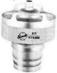
This Eimac tetrode is electrically identical to the 4CX5000A except for its plate dissipation rating and is intended for use where the extra plate dissipation is a necessity. It may be used at maximum ratings through 30 MHz and at slightly reduced ratings through the FM broadcast band.
