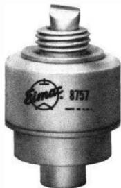
The 8757 is a miniature, ceramic and metal planar triode designed primarily for CW amplifier and oscillator application. This tube will also perform well as a grid or a plate-pulsed amplifier or oscillator at frequencies up to at least 3000 MHz.
