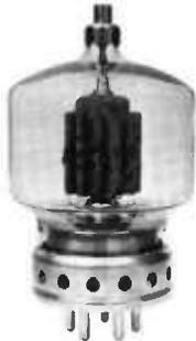
The 6580 is a 400-watt high-mu power triode designed especially for grounded-grid RF amplifier service, but is also capable of good performance in other applications. Because of its high amplification factor and high perveance, the 6580 will provide power gains as high as ten in grounded-grid amplifier applications. Because of internal shielding, neutralization is not required.
