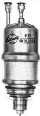
The 8173/4W20,000A is a high-power, water-cooled, power tetrode which will operate efficiently as a power amplifier at frequencies up to 250 MHz. A single 8173/4W20,000A operating as a television visual RF amplifier will deliver a synchronizing power output of 26 kW at 216 MHz with 5 MHz bandwidth. The coaxial construction of the tube is ideal for cavity circuits.
