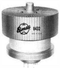
The 8432 is a ceramic-metal beam pentode featuring compact construction. The tube is especially suited for low-distortion Class AB<sub>1</sub> linear RF amplifier use where a single tube will deliver over 1500 watts of useful power output. The tube also provides outstanding performance in Class AB<sub>2</sub> and Class B service.
