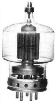
The 5-500A is a compact, ruggedly constructed radial-beam power pentode with a maximum plate dissipation rating of 500 watts. It is intended for use as an amplifier, oscillator or modulator. The high plate-current rating, low grid-plate capacitance and low driving power requirements permit maximum power capability to be combined with circuit simplicity and economic driver requirements.
