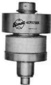
This tube is a pulse rated version of the coaxial 4CX250K. New cathode techniques permit pulse currents of over three amperes at pulse lengths up to 250 microseconds. Peak power output of 10KW is available at 0.005 duty.
