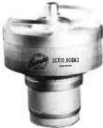
Here is a ceramic-metal medium-mu triode designed for industrial-heating oscillator service. It features a large thoriated-tungsten filament with ample reserve emission and an integral anode cooler with the inherent ability to withstand large overloads. It is intended for use through 140 MHz, also as a grounded-grid FM amplifier developing 20 kilowatts useful output power.
