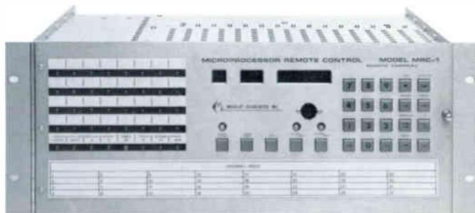
Microprocessor Remote Control System. Includes one Control Terminal and one Remote Terminal. Up to nine Remote Terminals function with a single Control Terminal. For 2-wire or 4-wire dedicated wireline or equivalent interconnecting circuits. Basic system equipped for 16 command lines (open collector electronic switching), 16 status channels (TTL/contact closure), and 16 telemetry channels indicated as 16/16/16. OPTIONS PRICES UPON APPLICATION.
