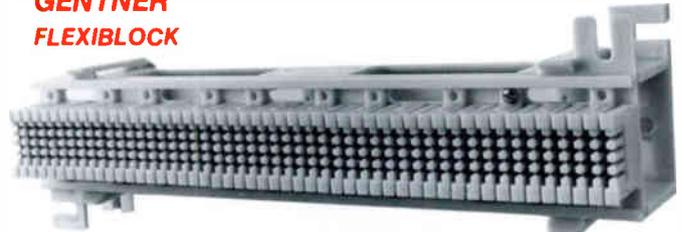
The Gentner Flexiblock is an insulation-displacement punch block system made specifically for stranded wire. Connections to Flexiblock are fast, easy and reliable. A high number of connections may be made in a small space (up to eight connections per circuit) and connections are virtually short-circuit proof. Standard size is 10"L x .56"H x 3.37"W with 50 terminals. (Variables available)
