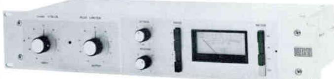
The UREI 1176LN single channel limiter features FET gain reduction ahead of the first stage. No tricky balancing required ever, there's no distortion adding active element in the gain reduction circuit, pushbutton selection of four different compression ratios and ultra fast attack time independent of peak duration or frequency and it's fully adjustable from the front panel.
