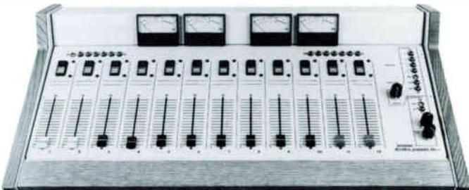
Designed for ease of operation, uncompromising performance and durability, is the 2000SC console. Each of the 12 channels features a single input per channel. Two remote select switches bring in an additional 14 inputs. Cue is accomplished by a detent on the industries finest fader while lighted momentary reed relay switches actuate the program and audition buses which are simultaneously monitored with VU meters. What console could be more rugged in
