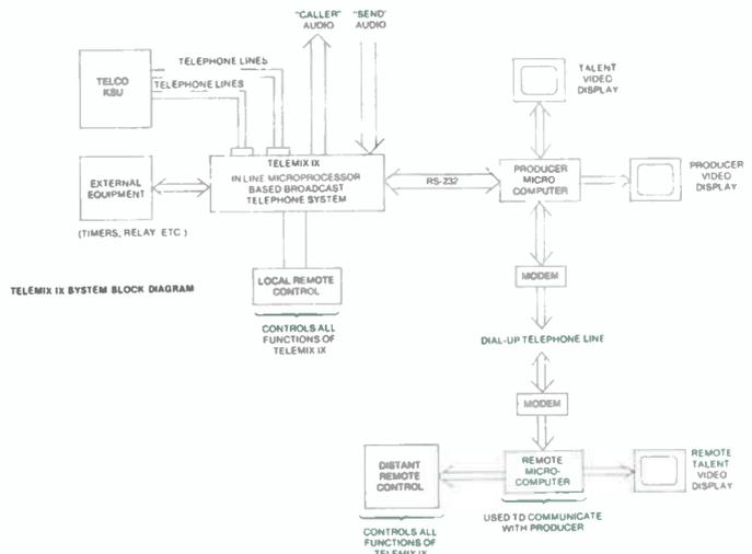
In summary, TELEMIX IX is a software driven, microprocessor based, multi-line telephone system that provides high quality telephone audio. The system is software driven, allowing maximum flexibility in processing telephone lines. The RS-232 port permits long distance remotability and in-house programming via a minicomputer. The system uses an advanced design telephone hybrid that produces clean, clear audio.
