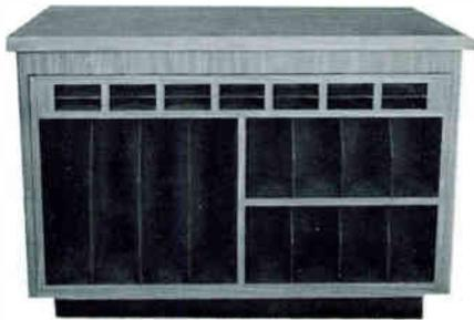
A-LINE turntable bases are constructed of 3/4" high-density particle board covered with standard laminates. Tops are 1 1/4" thick. Turntable bases are normally supplied with rack rails constructed of 11 gauge steel, tapped to accept 10-32 standard EIA rack panel screws. Cover panels are available at \$6 per bay. Custom cabinets with record and/or tape storage inserts are available.
