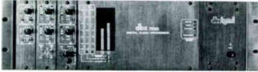
Precision Companding solves a major problem with delta modulation—limited dynamic range. The dbx 700 offers a dynamic range of more than 110 dB, resulting in an unbelievably low noise floor that's completely neutral-sounding. The compander's novel design and the direct digital link between encoder and decoder guarantee its overall performance is absolutely transparent.
