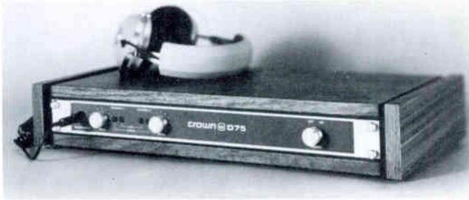
The CROWN D-75 offers significant benefits to the professional user, benefits like IOC input/output comparator that reports all forms of signal overload, lockable level control shafts, active-balanced XLR connectors as well as unbalanced 1/4" phone plugs and signal presence indicators that notify the user whenever the D-75 output signal is greater than 1/8 watt. 35 watts per channel.
