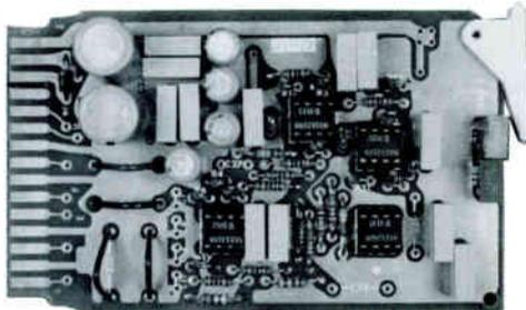
The MTX-2 allows you to optimize FM stereo coverage without smashing the audio. The reason heavy audio processing improves coverage is because of its effect in stereo. Stereo FM's coverage is sensitive to processing because the L-R signal is an AM suppressed carrier, double side band signal which makes the receiver sensitive to AM noise. Just turning on the stereo generator
