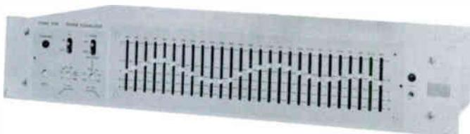
The Model 539 is an active filter set specifically designed for room "equalization" or tuning. The 539 utilizes advanced circuit technology and latest state-of-the-art components to achieve quantum improvements in performance and at lower cost. Signal to noise ratio is better than 110 dB at maximum output. Filter parameters have been optimized to produce excellent combining and minimum phase shift.
