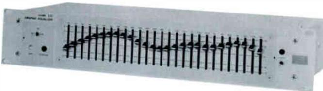
The Model 537 is a 1/3 octave equalizer set for general purpose frequency response adjustment of audio signals. It offers 27 adjustable equalizers on ISO 1/3 octave center frequencies, 12 dB boost or attenuation at each center frequency, stepless-noiseless controls, precision calibrated, state-of-the-art L-C filter circuitry, low distortion-low noise with minimum phase shift, zero insertion loss and is rack-mountable.
