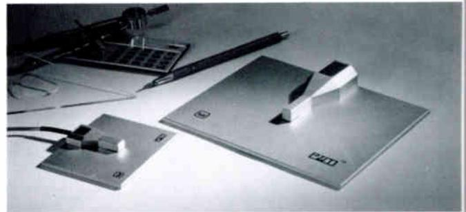
The pressure recording process, invented by Long and Wickersham, introduced a bright new concept to audio engineering. They discovered that sound approaching a boundary such as a floor, wall, table, podium, etc. creates a thin zone in which the direct and reflected signals are coherently in phase and reinforce each other. The Crown PZM microphone creatively realizes the potentials of that invention offering significant improvements in signal clarity and range. Comb filtering is eliminated.
