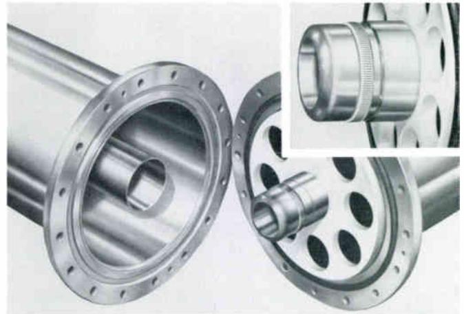
Comark rigid coaxial transmission line provides outstanding features such as constant impedance, high power capacity, and low insertion loss. Sizes to 8 3/16" Heliarc-welded flanges and wrist band bullet construction 3 1/8" and above.
