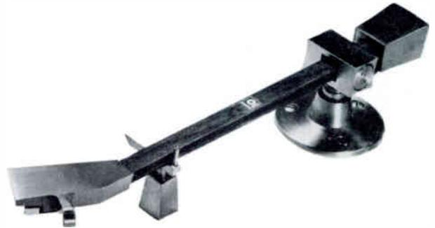
This tone arm features modern styling, plug-in memory balance head; laminated wood and epoxy body make for rugged, lightweight construction. Stylus force once set is tamper proof, and adjusted by counter-weight. A standard of the industry.
