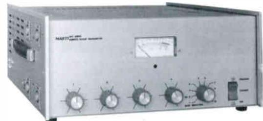
The Model RPT-25 transmitter provides uncompromised performance in portable and mobile remote broadcast service. This transmitter delivers 25 watts output under continuous duty conditions. Plug in modular construction simplifies field repairs. Available in dual frequency model. (RPT-40 delivers 40 watt output.)
