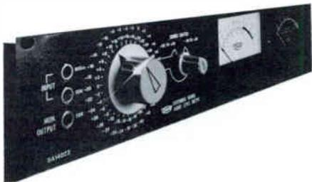
The SA14023 extended range audio level meter is a self contained instrument designed for the measurement of peak and average audio system transmission levels in dBm. A two position range switch and precision attenuator allow the accommodation of audio input levels from -50 dBm to +30 dBm, in 2 dB steps, for a zero meter reading (sine wave).
