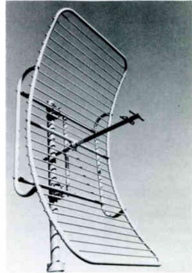
The Scala PR-450-U™ is widely used in point to point communications and telemetry systems in the 350 to 1000 mHz spectrum. Paraflector™ performance approximates that of a parabolic dish of the same aperture, and is easier to assemble and install. The PR-450U offers rugged construction for reliable long-term service, even in severe environmental conditions.
