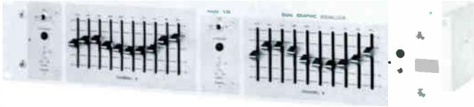
The UREI 535 dual graphic equalizer offers 10 filter sections per channel with increased control range, and more output capability. The 535 provides 12 dB of boost or cut at each of its 10 frequencies, which are centered at ISO one-octave increments from 31.5 Hz to 16 kHz, with balanced bridging differential amplifier inputs, variable gain, floating transformer isolated outputs of 150 ohms or greater load and is rack-mountable.
