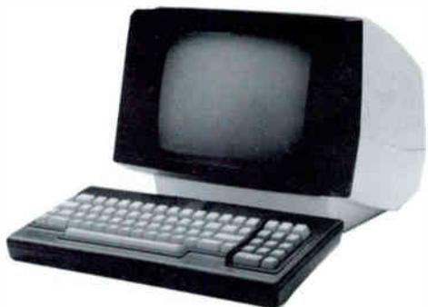
Option for cathode-ray tube (CRT) Terminal. Duplicates all panel functions of the MRC-1600 Control Terminal. Allows simultaneous display for 16 channels, including telemetry readings, status conditions, time of day, operation and error-oriented messages.
