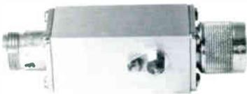
The **Allied Power Inserter/D.C. Block** is used as a power inserter for supplying external bias to an LNA independently of the satellite receiver. When used as a D.C. Block, multiple receivers can be connected to one LNA and only the desired LNA power be allowed to pass from the desired receiver. Type "N" connectors are standard.
