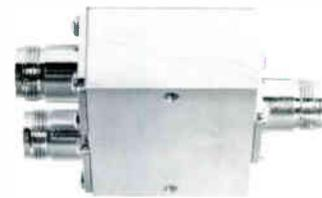
The **Allied PD-2 Series of Power Dividers/Splitters** are employed to divide an RF input signal in the 3.7-4.2 GHz (C-Band) satellite band. Two-way split, rugged construction, female type "N" connectors, D.C. passive are standard features.
