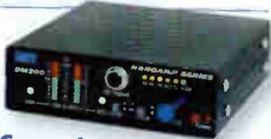
The NanoAmp DM200 DAC is a high-performance 24-bit/96 kHz digital-to-analog converter. Digital input formats include AES/EBU and S/PDIF via 110 Ohm XLR, 75 Ohm BNC and RCA connectors. It features transformer-isolated inputs, digital and analog stereo LED meter, stereo headphone and balanced audio outputs. 1/3 RU enclosure. Requires power supply (ATI wall mount supply listed below).
