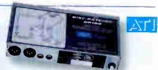
The ATI DP100, a unidirectional stereo interface, converts the unbalanced IHF outputs of CD players to transformer-balanced and isolated 600 ohm line levels with no compromise or degradation of the source audio. Optional rackmount kit available (holds two units). The MM100 is a bi-directional version.
