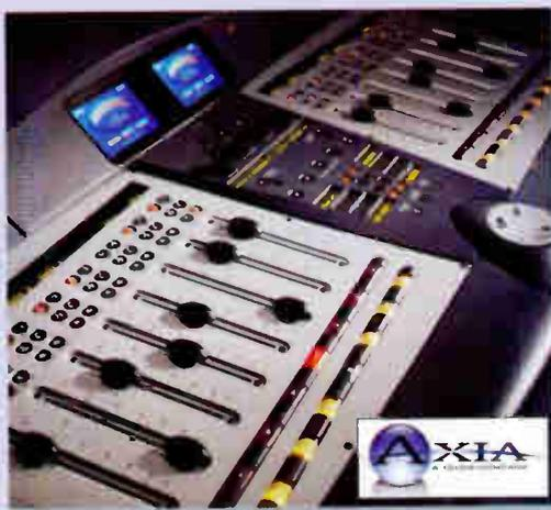
That's right... Ethernet. A 100Base-T segment, using a standard CAT-6 cable, can carry 25 stereo channels of 48 kHz, 24-bit linear PCM audio in both directions; a 1000Base-T link or Gigabit fiber can carry hundreds of channels. Segments are connected using modern Ethernet switches to enable a single network to carry in excess of 32,000 stereo channels! All for about half the cost of a traditional hardwired routing switcher.
