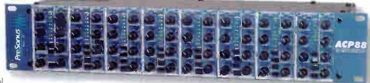
The PreSonus ACP88 is an 8-channel processor. Each channel provides crystal clear, musical compression and is equipped with full-featured controls including variable attack and release and soft/hard knee.
