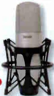
Shure's KSM32 is an externally-biased, dual large diaphragm cardioid condenser mic with extremely low self-noise (7 dB). It features a cardioid polar pattern, dual 1-inch, externally biased diaphragms, a Class A, discrete, transformerless preamp, a subsonic filter, a 15 dB pad switch, 3-position switchable low-frequency filter, integrated three-stage pop grille and internal shockmount. Includes shockmount, swivel mount and case.
