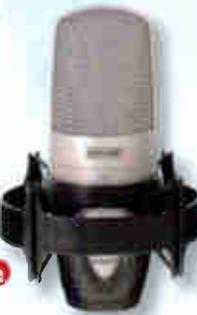
The KSM27 side-address condenser delivers Shure reliability and outstanding sound at a bargain price. It has a cardioid polar pattern; 1-inch, externally biased diaphragm; Class A, discrete, transformerless preamplifier and a subsonic filter which eliminates rumble below 17 Hz. Other features include a switchable 15 dB pad; 3-position, low-frequency filter; internal shockmount and an integrated three-stage pop grille. Includes elastic shockmount and case.
