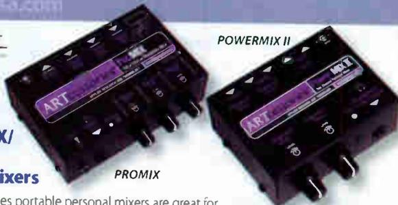
ART's ProMIX Series portable personal mixers are great for adding extra sub-mixable inputs to larger mixers thru 1 or 2 channels. The ProMIX is a 3-channel mic mixer with switchable 12V phantom power and low-frequency cut on each channel. Output is via mono balanced XLR and a headphone/aux 1/4" jack. It's powered by an included 12V AC adaptor or two 9V internal batteries.
