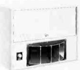
ALTEC 844A MONITOR & PLAYBACK SPEAKER SYSTEM was designed especially for convenient use in studios. Contains two 12" LF speakers and 800-Hz horn with driver and dividing network. Horn is positioned below the LF speakers so that entire unit may be mounted above the observation window. Provides exceptionally smooth frequency response from 30 to 22,000 Hz. Only 24"H x 31"W x 16"D.
