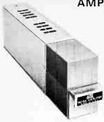
ALTEC 9470A AMPLIFIER can serve as preamp, line, booster, or program amplifier with no internal changes. All-silicon transistor circuitry delivers 0.5 watt and may operate continuously at 85°C without derating. Frequency Response: ±0.5 db, 20-20,000 Hz. Less than 1% THD, 20-20,000 Hz, with +27 dbm out-
