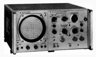
**140A** – Oscilloscope with 1415A Time Domain Reflectometer Plug-In
