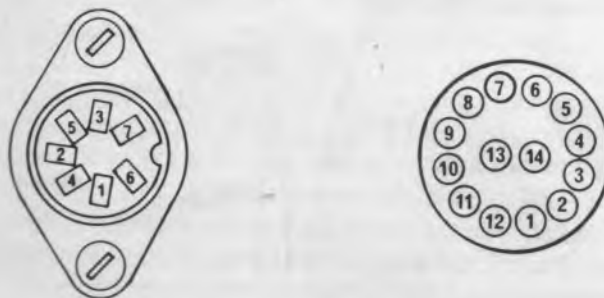
FIG. 15. REMOTE AND AUXILIARY SOCKET CONNECTIONS
