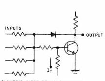
(a) CLAMPING DIODE REDUCES STORAGE TIME TO INCREASE SPEED
