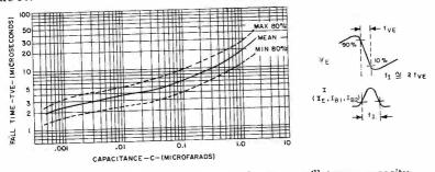
Recovery time of unijunction transistor relaxation oscillator vs. capacity FIGURE 90
