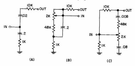
(A) A I KC EQUIVALENT CIRCUIT. (B) LOW - FREQUENCY EQUIVALENT CIRCUIT, AND (C) THE EQUIVALENT CIRCUIT AT HIGH FREQUENCIES.
