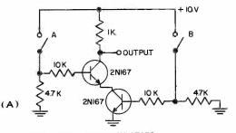
GATE USING NPN TRANSISTORS IF CLOSING A SWITCH IS AN INPUT THIS IS AN "AND" GATE IF OPENING A SWITCH IS AN INPUT THIS IS AN "OR" GATE NOTE: PHASE INVERSION OF INPUT
