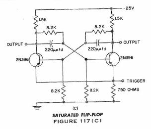
The circuit in Figure 117(c) is stabilized to  $100^{\circ}$ C. The price that is paid for the stability is (1) smaller voltage change at the collector, (2) more battery power consumed, (3) more trigger power required, (4) a low I<sub>co</sub> transistor must be used. The capacitor values depend on the trigger characteristics and the maximum trigger repetition rate as well as on the flip-flop design.
