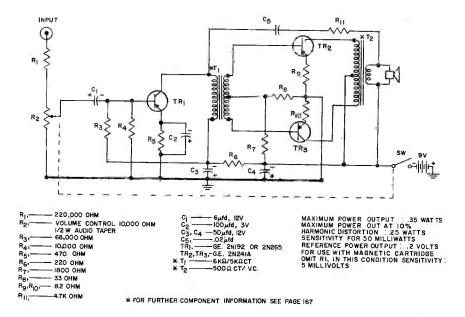
THREE TRANSISTOR PHONO AMPLIFIER FIGURE 41 BASIC AMPLIFIERS
