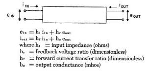
For transistors, a second subscript is added to designate which terminal of the transistor is grounded. For example,  $h_{fe}$  is the grounded emitter forward current transfer ratio.
