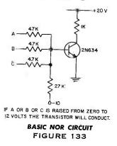
"NOR" logic is a natural extension of the use of resistors in the base circuit. In the circuit of Figure 133, if any of the inputs is made positive, sufficient base current
