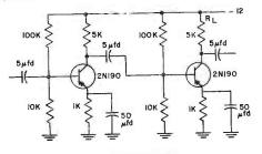
The load resistance for the first stage is now the input impedance of the second stage. The voltage gain is given approximately by the formula:
