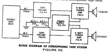
Two identical tape preamplifier circuits can use a common 18 volt battery supply. The circuitry of Figure 44 may be used with the switch and RIAA network eliminated if the preamps are to be used for tape only.
