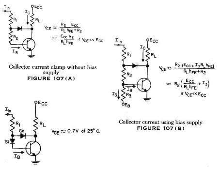
Collector current clamp using silicon and germanium diodes FIGURE 107 (C)
