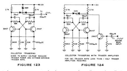
In designing a counter, it may be advantageous to design all stages identically the same to permit the economies of automatic assembly. Should it prove necessary to increase the speed of the early stages, this can be done by adding a trigger amplifier as shown in Figure 124, without any change to the basic stage.
