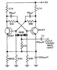
BASE TRIGGERING MAXIMUM TRIGGER RATE EXCEEDS I MC WITH TRIGGER AMPLITUDE FROM 0.75 TO 3 VOLTS.
