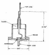
over 1/4 ampere at room temperature and block voltages in the reverse direction up to 300 volts peak. This latter rating is called the "Peak Inverse Voltage" of the cell. When this same cell is mounted on a 1-1/2 inch square fin as shown in Figure 17, its current carrying capabilities are increased to over 3/4 ampere at room temperature.
