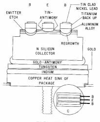
By using two impurities diffused simultaneously, it is possible to form a P type layer .2 mil thick and an N type emitter layer .3 mil thick. By making contacts to the base and emitter regions, a transistor is produced capable of carrying up to 10 amperes. Since the diffused layers are very thin, the frequency response of this power transistor is good up to 5 to 10 mc.
