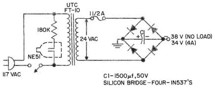
POWER SUPPLY FOR DUAL SIX-WATT AMPLIFIER FIGURE 154
