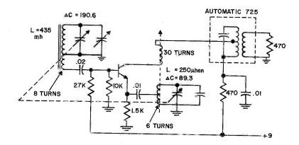
ANTENNA - DELTA COIL # I - 105A OR EQUIVALENT OSCILLATOR COIL - E. STANWYCK CO. # 1129 (MODIFIED) OR EQUIVALENT CAPACITOR - RADIO CONDENSER # 242 OR EQUIVALENT I. F TRANSFORMER - AUTOMATIC 725 (EXO-3926) OR EQUIVALENT
