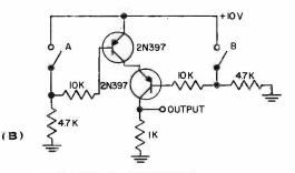
GATE USING PNP TRANSISTORS IF CLOSING A SWITCH IS AN INPUT THIS IS AN "OR" GATE IF OPENING A SWITCH IS AN INPUT THIS IS AN "AND"GATE NOTE: PHASE INVERSION OF INPUT
