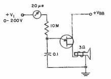
TEST CIRCUIT FOR INTRINSIC STANDOFF RATIO (7)
