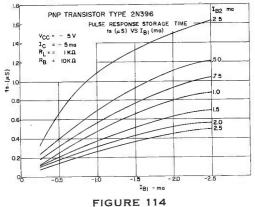
an unsymmetrical transistor with the same  $h_{FE}$  and  $f_{\alpha}$ . Figure 114 shows the dependence of storage time on  $I_{B1}$  and  $I_{B2}$  for the 2N396 transistor.
