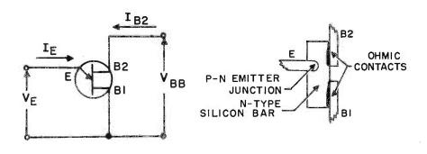
Symbol for unijunction transistor with indentification of principle voltages and currents FIGURE 80 Construction of unijunction transistorcross sectional view
