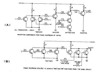
Circuits representing  $(I + M + L) (\overline{I} + M + \overline{L}) (\overline{I} + \overline{M} + L) = \overline{R}$ FIGURE 132
