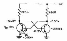
DIRECT COUPLED TRANSISTOR LOGIC (DCTL) FLIP-FLOP FIGURE 105
