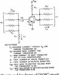
Circuit used for design of "NOR" circuitry FIGURE 135 A detailed "NOR" building block is shown in Figure 135. The figure defines the basic quantities. The circuit can readily be designed with the aid of three basic equations. The first derives the current  $I_{\kappa}$  under the worst loading conditions at the collector of a stage.
