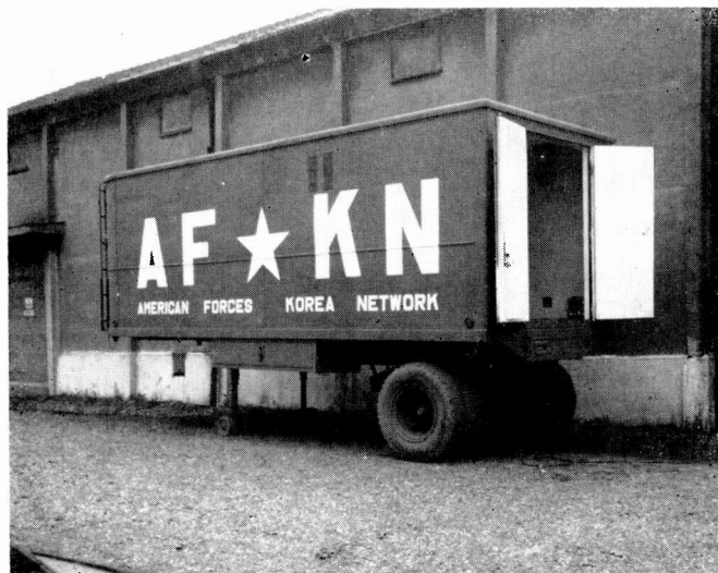
Indicating the rugged construction of the BC-1F transmitter is this mobile installation of the Armed Forces Korea network mounted in a six ton semi trailer van. Note the transmitter is firmly secured to floor with no snubbing connection to ceiling.
