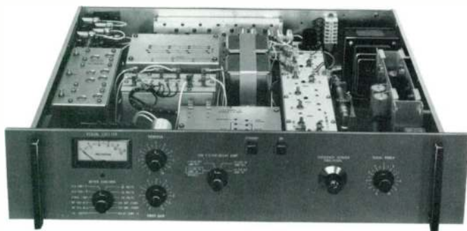
VISUAL EXCITER. Complete, self-contained one-watt, "on channel" signal source. Totally solid state. Modular construction.
