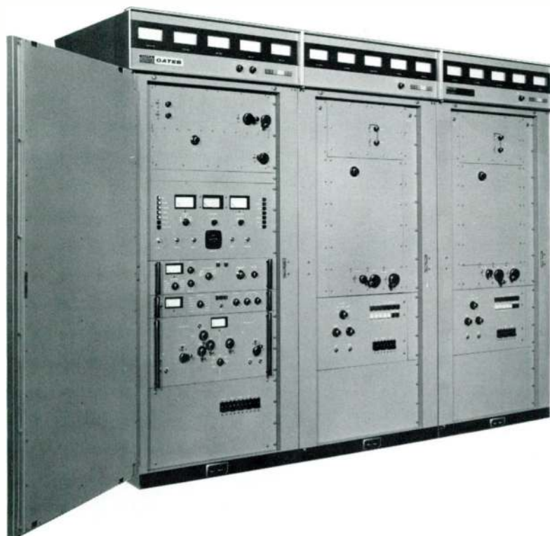
Front view, BT-18L, 18 kW low band transmitter, showing from left to right, the 1300-watt exciter/driver, the aural power amplifier and the 18 kilowatt visual power amplifier.
