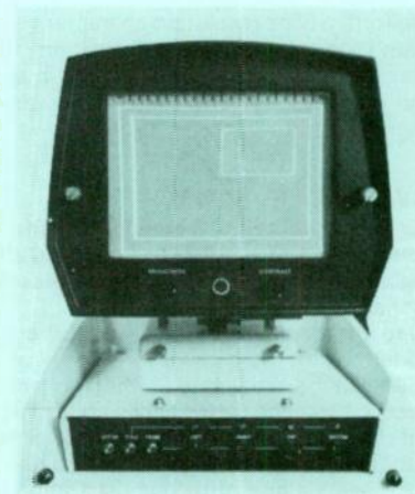
Operator's view of Harris C Series tiltable, rotatable viewfinder showing electronic-generated safe-title area and variable grease pencil window.
