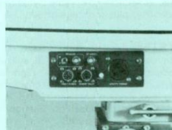
Utility panel provides connections for test equipment and external intercoms, tallies, monitors.
