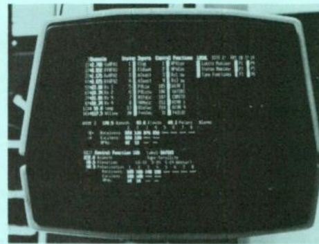
One of 24 CRT displays available on command, which gives detailed status information on earth satellite parameters.
