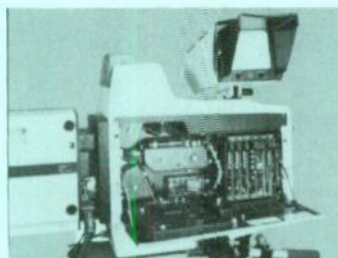
Camera-head modules are readily accessible for servicing, and controls are front-edge mounted.
