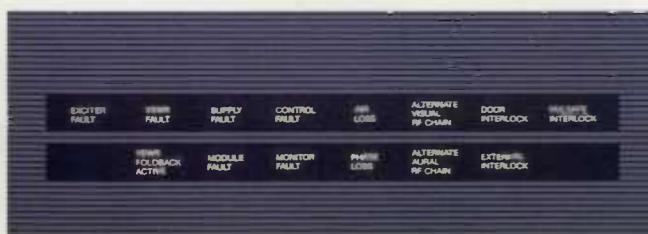
Status lights on the control panel illuminate automatically to indicate fault conditions.
