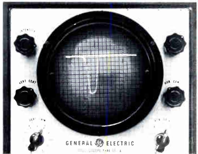
FIG. A-11. Normal alignment curve with the sweep width control in position #7.
