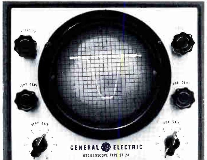
FIG. A-9. Normal alignment curve with the sweep width control in position #5.
