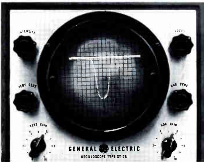
FIG. A-10. Normal alignment curve with the sweep width control in position #6.
