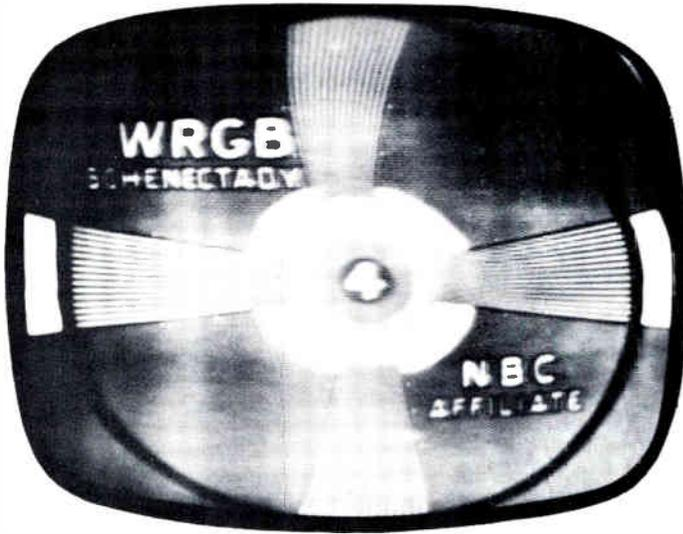
FIG. L-4. The shading of the test pattern is due to an open filter capacitor C453 in Figure L-5 which allows some a-c to modulate the video signal. The wave is due to a-c getting into the horizontal circuit.
