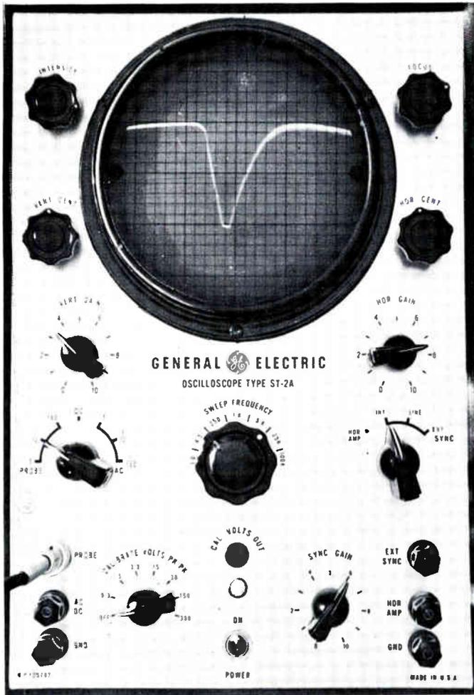
**FIG. I-10. Waveform at point 1 due to the same defect as I-9 but with the picture synced so that the blanking bar cannot be seen.**
