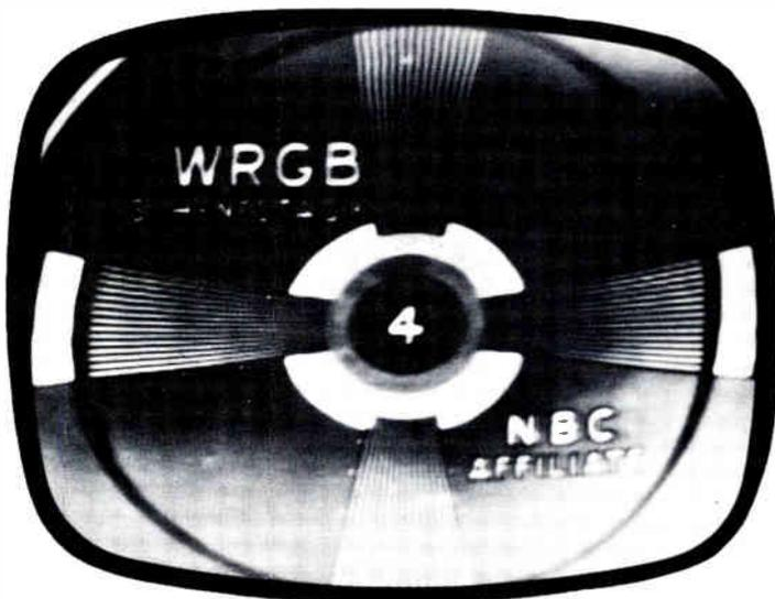
FIG. L-2. Test pattern with dark band due to heater-cathode leakage in one of the video i-f amplifiers.
