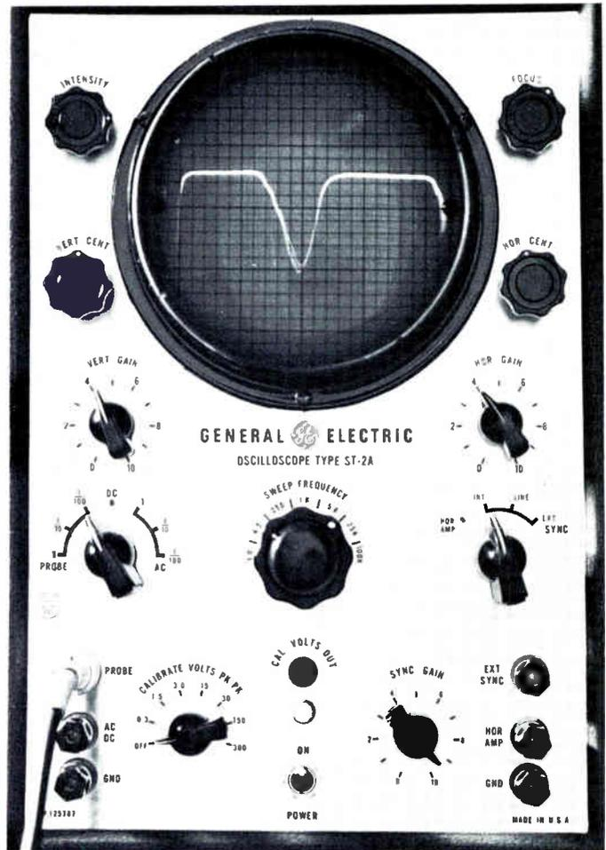
FIG. K-11. Waveform at point 2 in Figure K-1 with resistor R366 open. The amplitude is reduced to about 180 volts.
