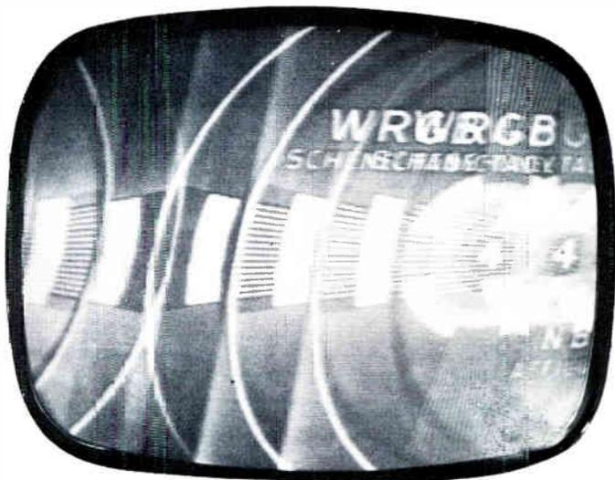
FIG. I-4. Test pattern as it appears with capacitor C356 open.
