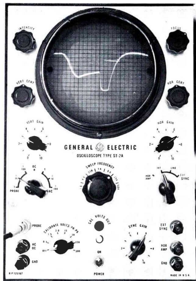
FIG. I-9. Waveform at point 1 due to leakage in capacitor C357 in Figure I-1. The picture is synced with the blanking bar at the left of the picture as shown in Figure I-7. The peak-to-peak voltage is about the normal 30 volts.
