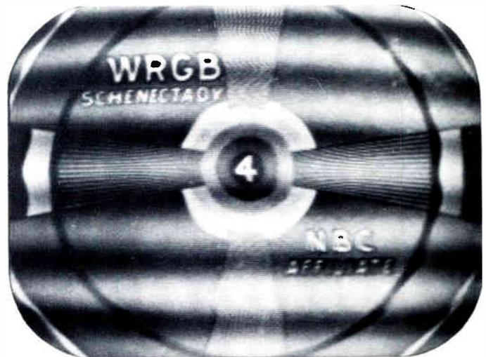
FIG. C-9. Test pattern with picture distorted by the sound carrier as shown in Fig. C-8 alignment curve.
