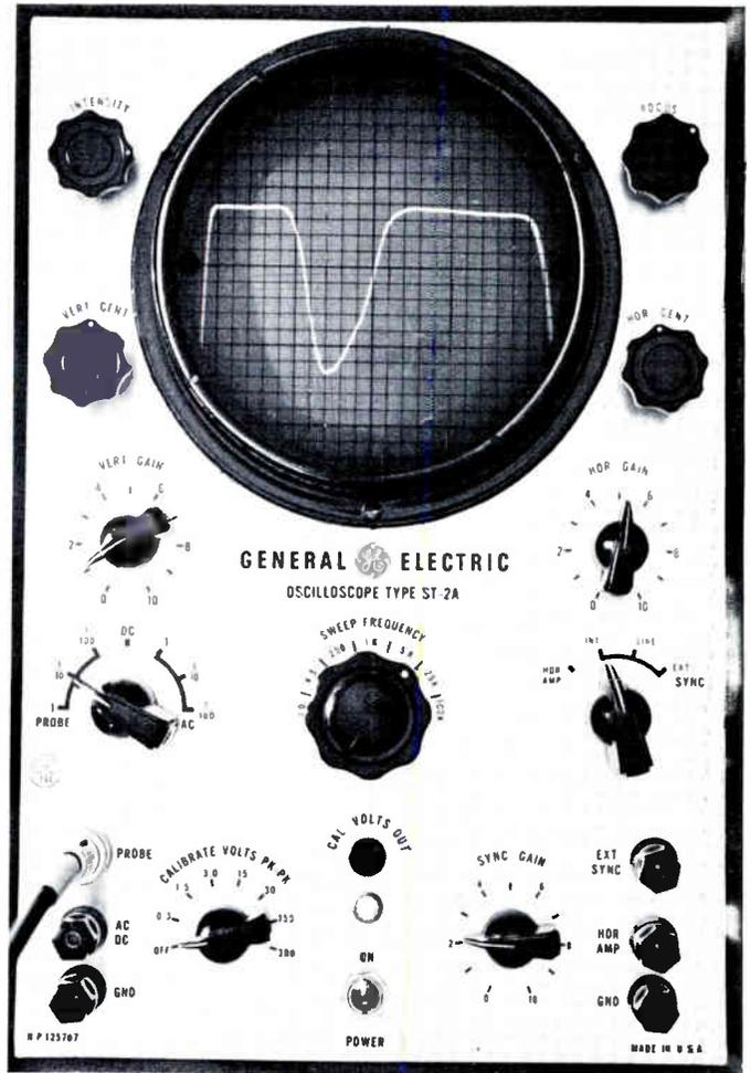
FIG. K-7. Normal waveform at point 2 in Figure K-1 which has a peak-to-peak voltage of about 210 volts.
