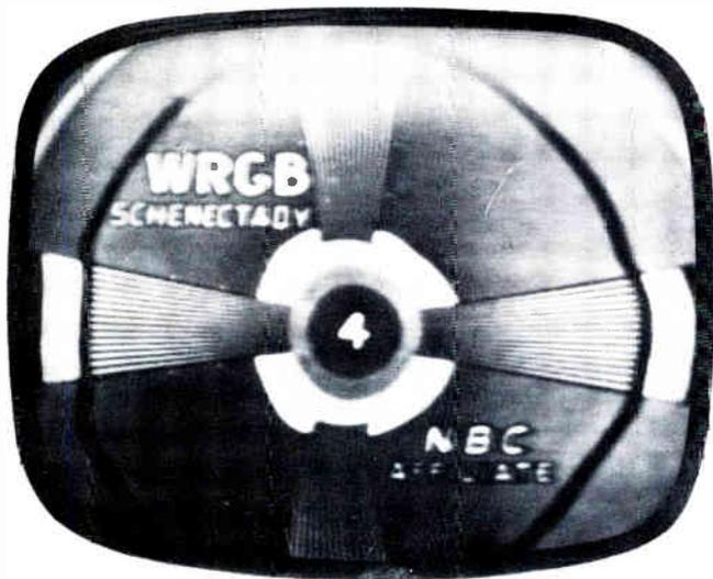
FIG. E-2. Test pattern showing the affect of clipping in the r-f or i-f stages.
