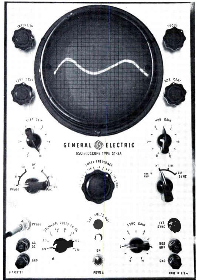
FIG. I-22. Waveform at point 3 due to a shorted capacitor C358. The peak-to-peak voltage is only slightly reduced to 0.5 volts.
