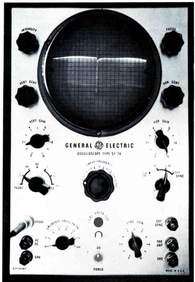
FIG. H-2. Normal vertical sync pulse at point 1 in Figure H-1.
