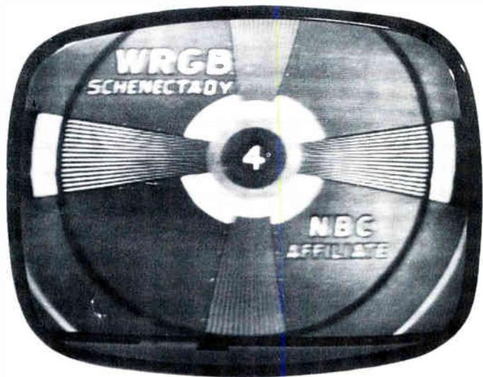
FIG. F-7. Test pattern showing the effect of an open capacitor C379C in Figure F-2.
