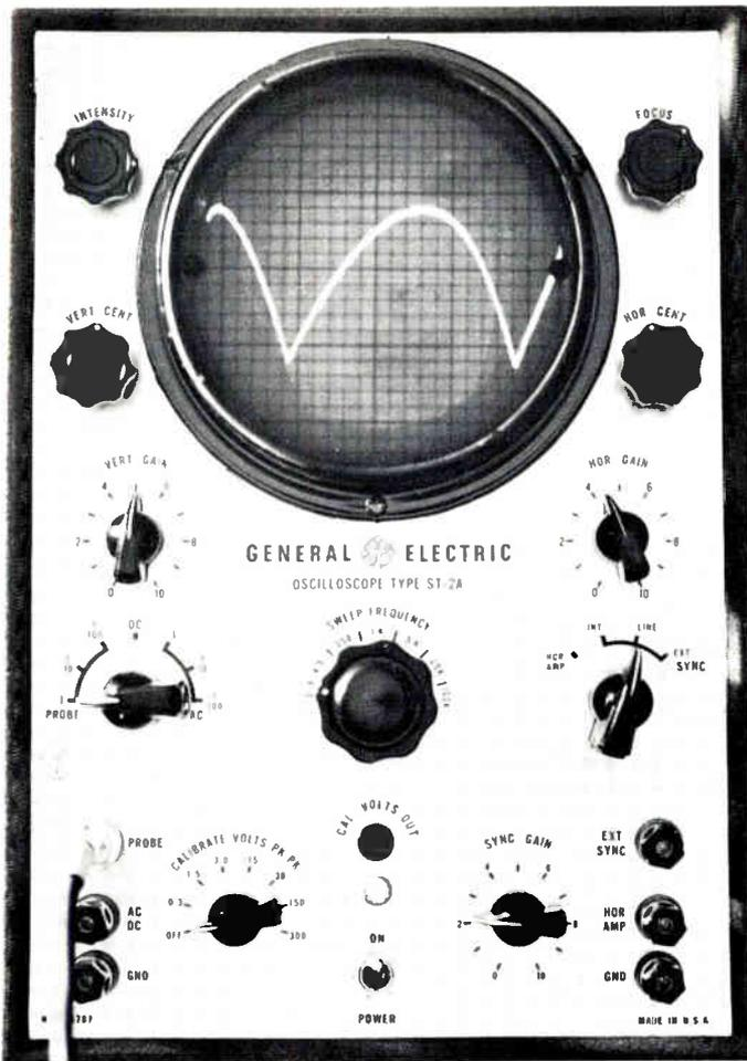
FIG. L-17. Normal waveform across capacitor C310 on the complete schematic shown on pages 28 and 29. Capacitor C310 is connected to the B side of the vertical sweep output transformer. The waveform at this point has a peak-to-peak voltage of about 2.0 volts.
