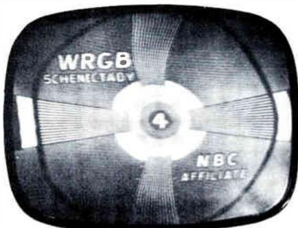
FIG. I-25. Test pattern due to a reduction in the value of R362 to 2K ohms.
