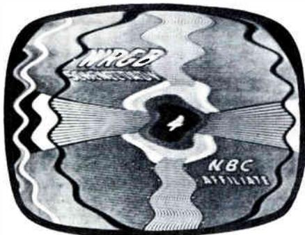
FIG. I-24. Test pattern due to open capacitor C375 in Figure I-1.
