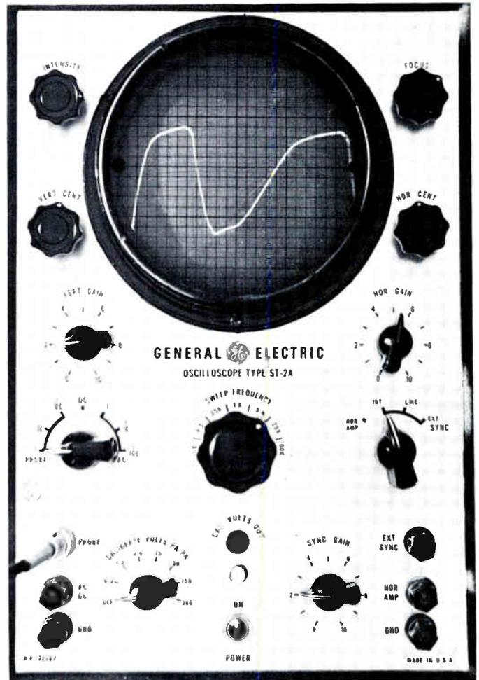
FIG. I-15. The waveform at point 3 is changed in shape and amplitude due to an open capacitor C361. The peak-to-peak voltage is increased to about 10 volts.
