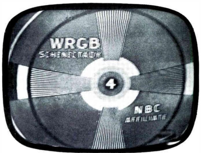
FIG. K-10. Distorted test pattern due to an open resistor R366.
