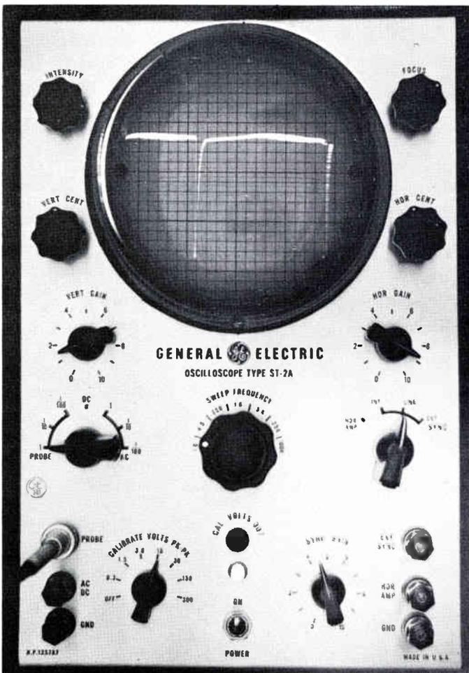
FIG. H-5. Waveform at point 2 in Figure H-1 with 100K leakage across capacitor C302.
