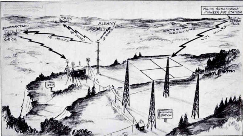
FIG. 2. HIGHER UP THE MOUNTAIN IS THE RELAY RECEIVING ANTENNA, USED TO PICK UP PROGRAMS FROM ALPINE. STUDIO-TO-TRANSMITTER LINK IS SHOWN BY ARROW
