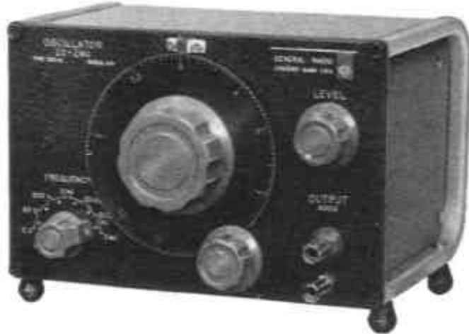
The Type 1310-A Oscillator, a descendant of GR's original 1938 R-C oscillator.
