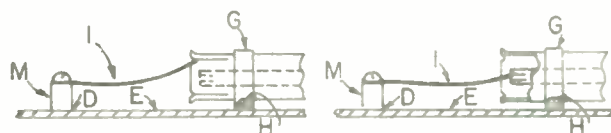
d. Short No. 20 bus wire used to measure input impedance to coaxial line. For initial balance, short inner and outer coaxial conductors by a strap, or connect bus wire to grounded shell of coaxial line. Most accurate method, especially at higher frequencies
