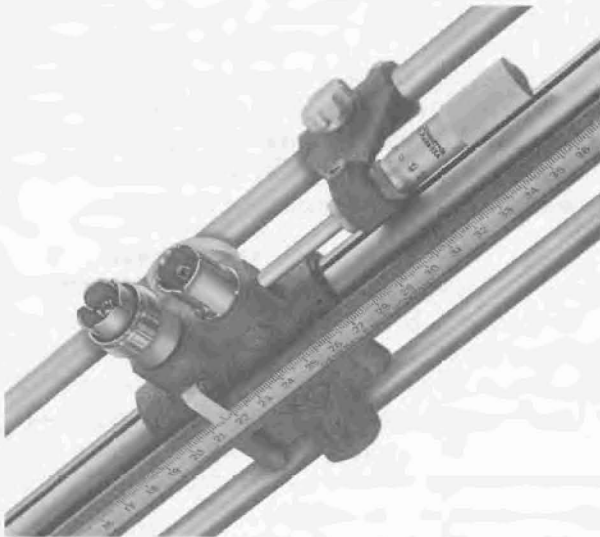
Figure 5.2-2. The slot along the top of the line's outer conductor is clearly visible in this close-up of the carriage assembly, which also shows the micrometer in position.
