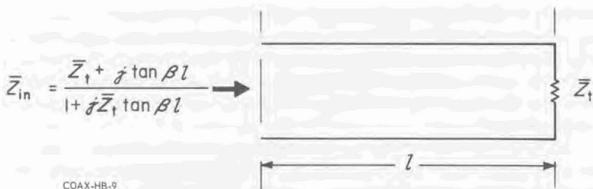
Figure 1.8-3. A transmission-line section of length l transforms the normalized terminal impedance \bar{Z}_t into a normalized input impedance \bar{Z}_{in} .
