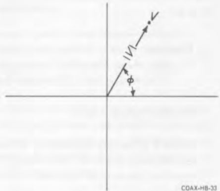
Figure 1.2-2. The phasor V = |V| \angle \phi .
