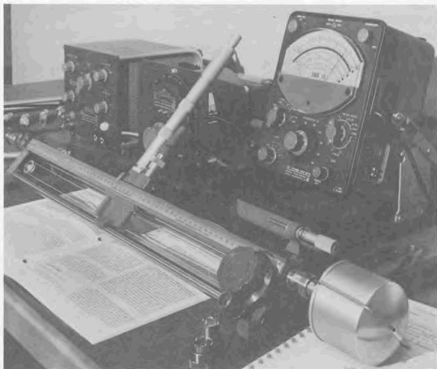
Figure 5.2-6. The General Radio Type 874-LBB Slotted Line with Type 900-DP probe-and-tuner and Type 1234 SWR Meter in a typical laboratory setup. Behind the slotted line on the left is the modulating power supply and next to it is the oscillator. The device under test is mounted in the shielded component mount attached to the right-hand end of the slotted line.
