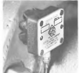
Vibration pickup with permanent-magnet clamp
