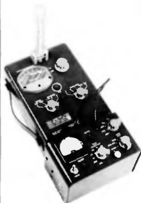
The 1556-B Impact-Noise Analyzer attaches to the 1551-C Sound-Level Meter as shown here.
