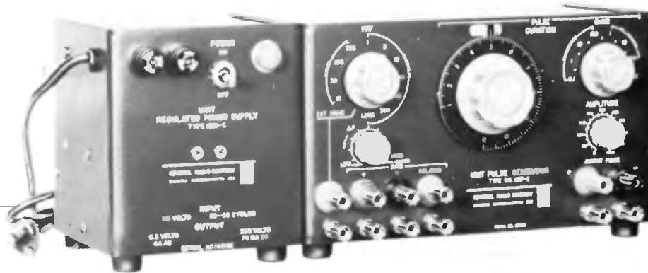
Unit pulse generator with power supply
