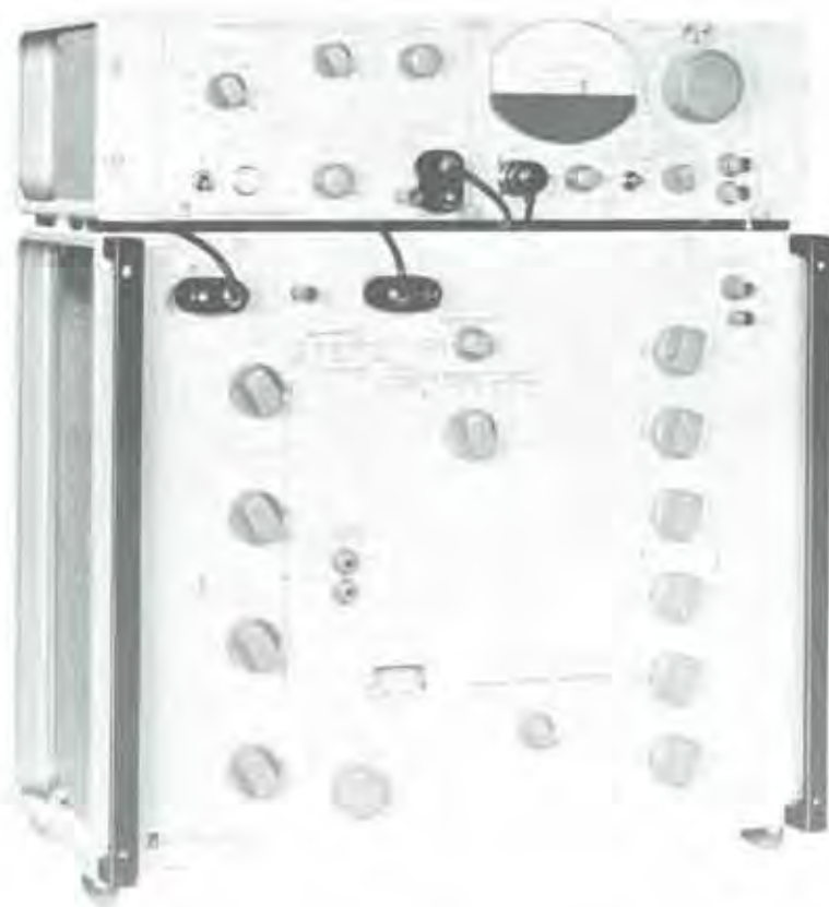
1660-A Precision Inductance-Measuring Assembly includes 1632-A Inductance Bridge, 1311-A Oscillator, 1232-A Tuned Amplifier and Null Detector.
