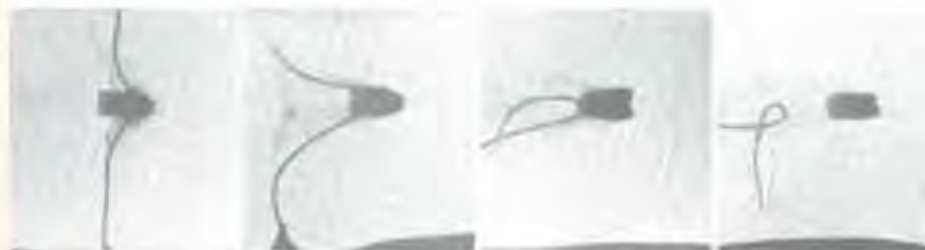
Strobe shadowgraph shows a .27 caliber bullet striking and being cut in two by a steel wire — the supersonic whip of the wire end is clearly visible. Separation of the four images is achieved by flashing the strobes at intervals of 40 microseconds.
