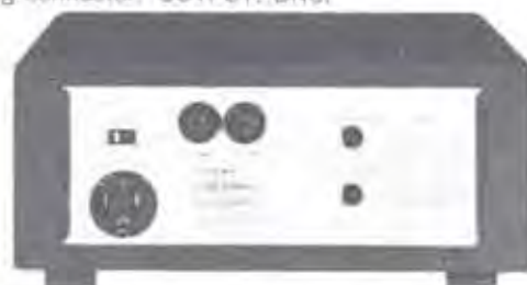
The input and output connectors can be moved to the rear for systems applications.
