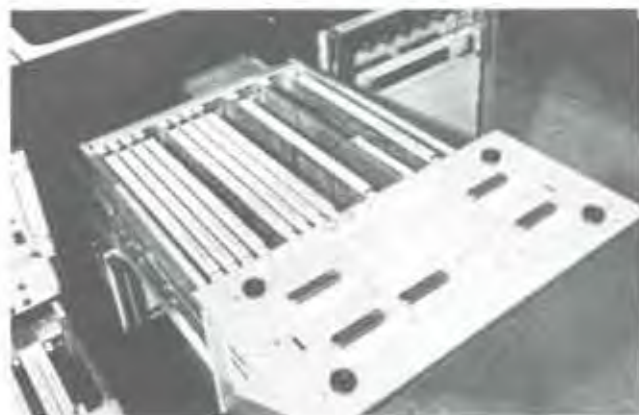
Computer-controlled scanner boards in Systems 2200.
