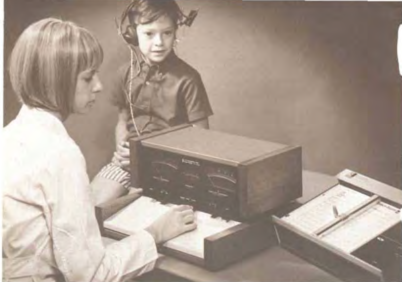
1720 Otoadmittance Meter as used in measurement of middle-ear function.
