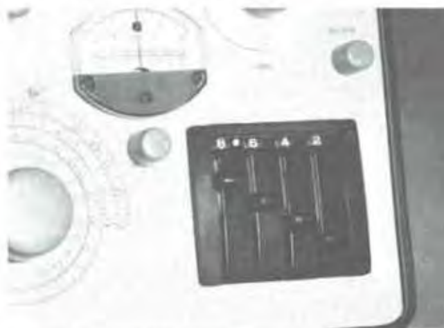
Lever-arm switches on 1656 permit fast balances and easy-to-read answers.
