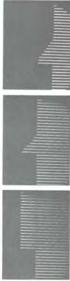
Oscillograms of line-voltage peaks show response speed of Variac® automatic voltage regulators: left, 2% step change in line voltage; center and right, resulting output transients for 1561 and 1562 Regulators, respectively.
