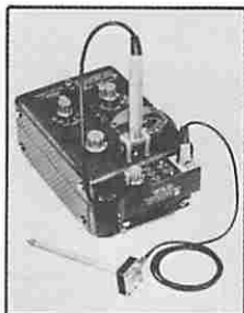
The 1560-P118 Vibration Pickup System with the 1551-C Sound-Level Meter.
