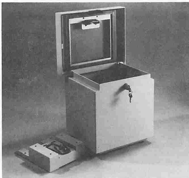
Figure 7-3. The vandal-resistant case for protection of the 1945 Community Noise Analyzer.
