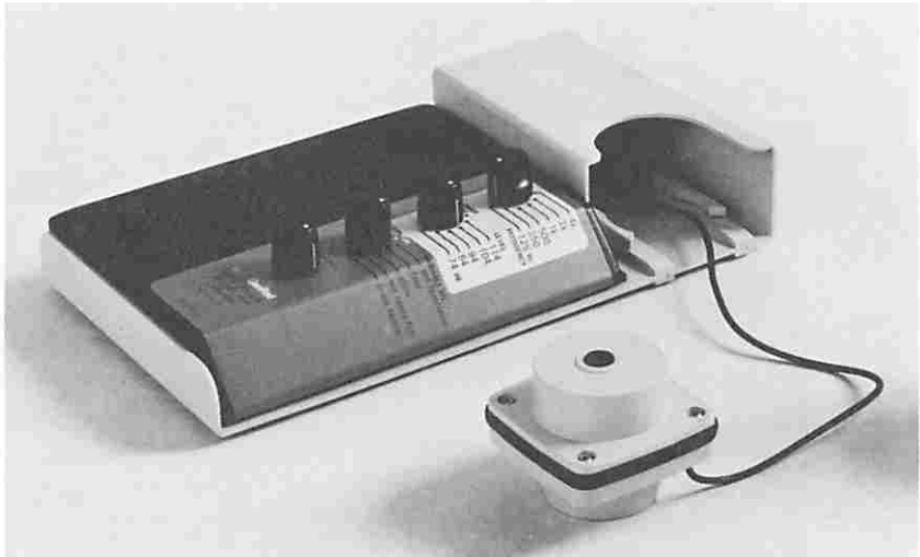
Figure 7-5. 1986 Omnical Sound-Level Calibrator.
