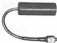
Figure 6-14. A typical hydrophone.
