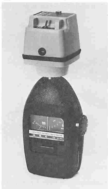
Figure 7-4. Type 1987 Sound Level Calibrator installed on a sound level meter.
