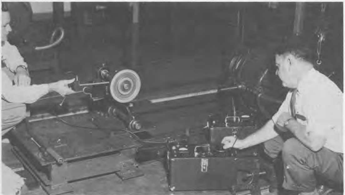
Figure 19. Shock-absorbing qualities of the Gates Super Rope are measured with the equipment shown here. Readings are taken at both the motor and the driven machine to determine how much vibration is absorbed by the belt.
