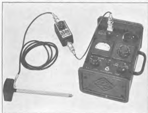
The vibration pickup and control box plug into the sound-level meter in place of the microphone, as shown in the photograph above.
