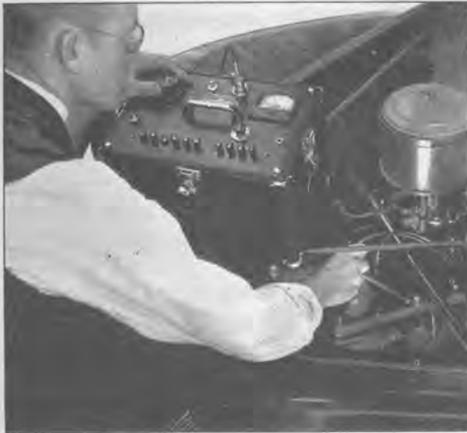
Measurement of automobile-engine vibration with the TYPE 761-A Vibration Meter.
