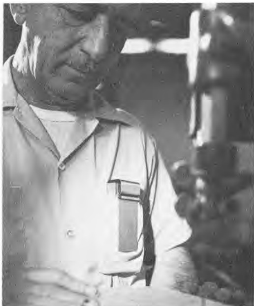
1. The GR 1944 Noise-Exposure Monitor, in worker's pocket, automatically measures noise exposure.
