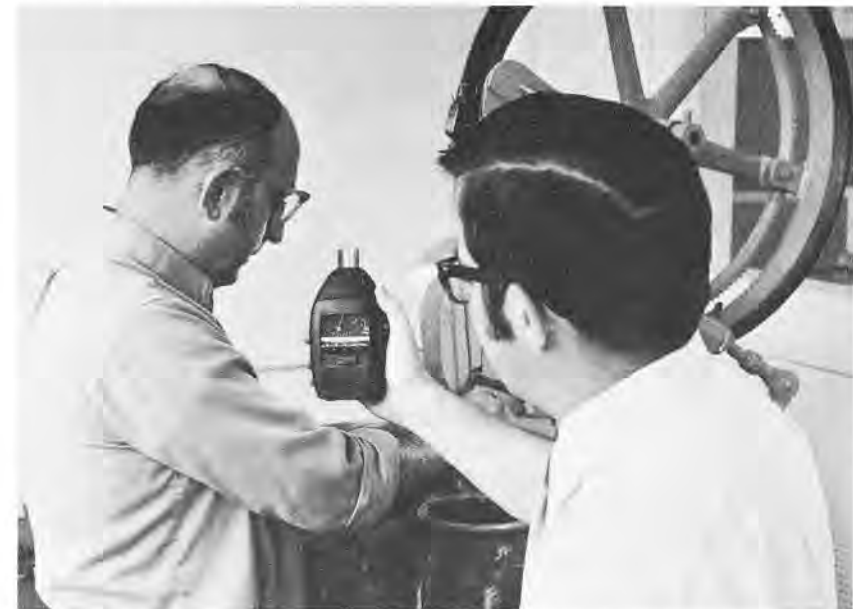
A plant-noise measurement made with the GR 1565 Sound-Level Meter.
