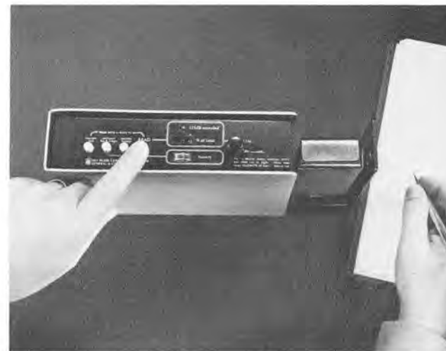
2. Monitor positioned on 1944 Noise-Exposure Indicator for read-out of accumulated noise exposure.
