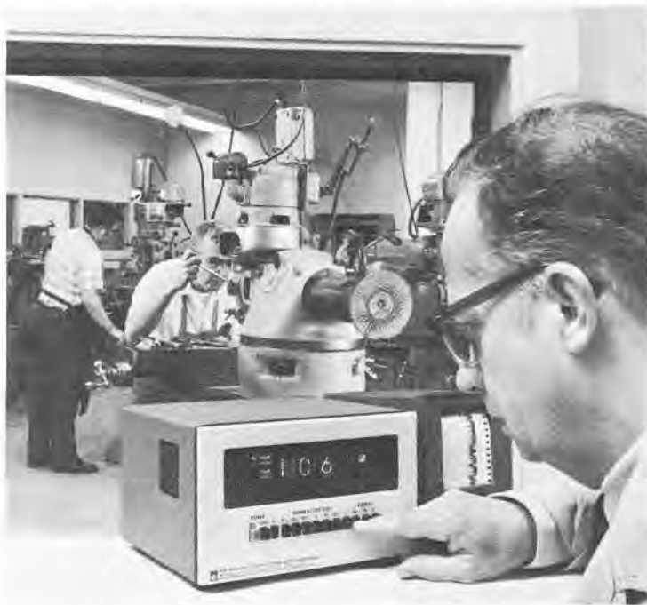
The GR 1934 Noise-Exposure Monitor, shown in an industrial application.
