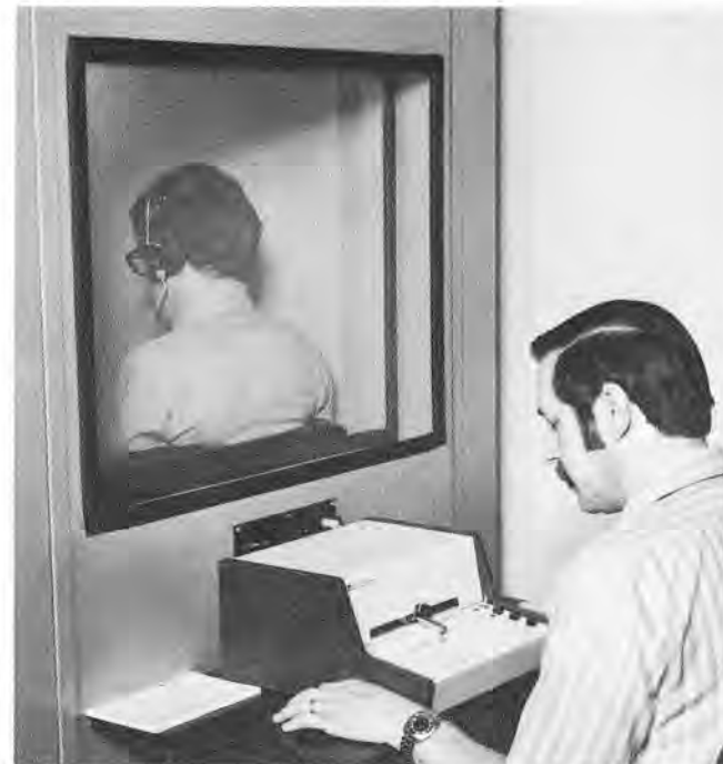
1703 Automatic Recording Audiometer, showing a freshly plotted audiogram of actual hearing-acuity response. The subject is seated in the GR 1939 Audiometric Examination Room.
