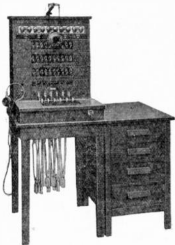
Method of Assembling No. 1800 Switchboard to 35 Line Capacity
