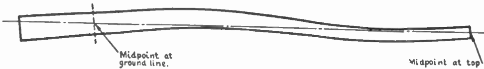
Diagram 2—Measurement of Sweep in 2 Planes (Double Sweep) or in 2 Directions in One Plane (Reverse Sweep)
