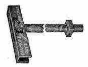
SECOND: Insert the nut through slot in sides of toggle head and turn the thread of stove bolt into the The toggle is then ready for use with a finished stove bolt head at the outside of the work exposed nut. o view.
