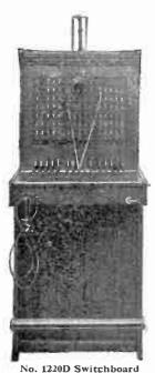
The No. 1200 type switchboard series (Code Nos. 1220 to 1259) is designed for the medium size magneto exchange. The switchboards range in capacity from 105 lines to 330 lines. Additional capacity may be obtained by lining up two or more sections and making use of transfer trunks.
