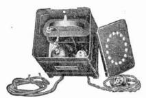
Interior View of 2 Ampere Tungar Rectifier
