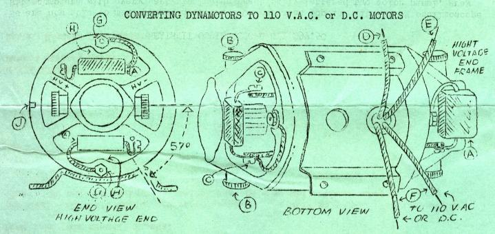
Many have requested this data. The type used is the DM-36 which we sell for \$1.50. To use as a motor, it is necessary to tap into the armature end and thread a pulley into the end, or have a shaft electric welded to the end. These dynamotors make excellent and powerful 110V motors.
