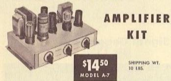
The Heathkit Model A-7 amplifier features beam power, push pull output with frequency response flat ± 1½ DB from 20 to 20,000 cycles. Separate volume, bass and treble controls. Two input circuits, output impedances of 4, 8, and 15 ohms. Peak power output rated at full 6 watts. High quality components, simplified layout, attractive gray finished chassis, break off type adjustable length-control shafts and attractive lettered control panel.
