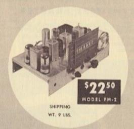
The Heathkit Model FM-2 Tuner was specifically designed for simplified kit construction. A pre-assembled and adjusted tuning condenser assembly, double tuned IF transformers and discriminator transformer and an 8 tube transformer operated circuit are among its many features. Smooth tuning is obtained through a 9:1 ratio vernier drive using a calibrated 6" alide rule type dial. Frequency coverage of 88 to 108 mc is provided. Kit supplied with all parts and manual.
