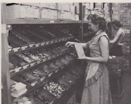
Individual small parts are selected from bins and packaged in bags for each kit.
