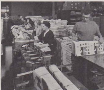
Stitching the catalogs two-up with six stations on an automatic stitcher.
