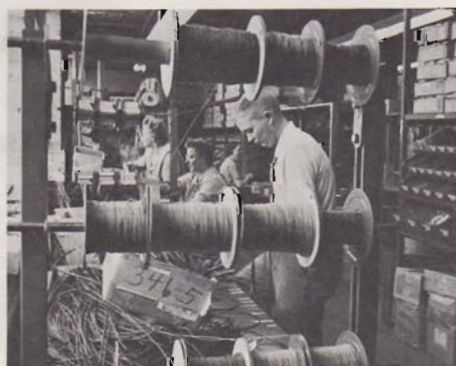
Various types of wire are taken from spools and cut to the proper length before packing.
