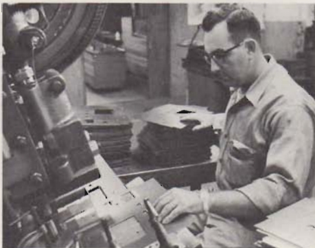
Sheet-metal work is done in our own factory. Here, a chassis is being punched.
