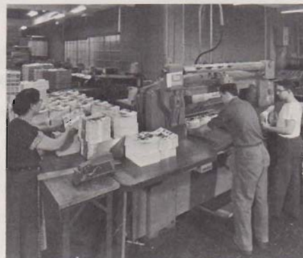
Cutting and trimming the catalogs is done on this cutter with an electronic spacer.
