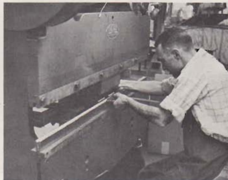
A machine is set up for chassis folding before a run is made.
