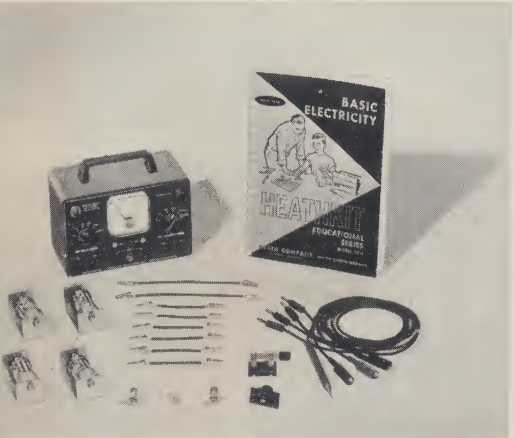
A KIT AND TEXT BOOK COMBINATION, the EK-1 includes all parts for experiments and you build a practical DC volt-ohm-milliammeter.
