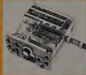
Exclusive Heath extender boards make test, adjustment and service fast and easy.
