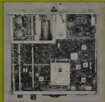
Clean, open chassis layout for easy assembly. Note completely shielded final, upper left.
