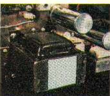
Transformer-operated power supplies
