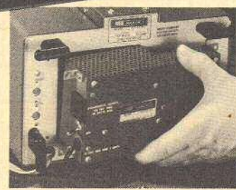
Optional power inverter mounts on rear panel for convenient on-the-road testing capability.
