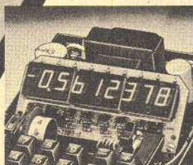
8-digit totals on bright 1/2" neon display tubes
