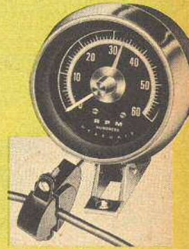
Inductive pick-up coil snaps easily into place on coil wire when points are inaccessible.
