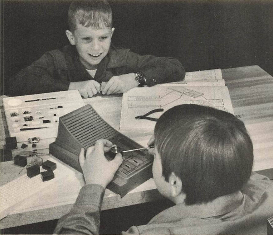
Actual components mount inside modules carrying the component's schematic symbol.
