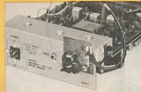
Crystal OSC/Mixer Signal Source simplifies alignment.
