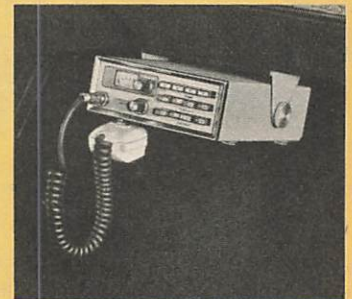
Neat mobile mount, supplied with your kit, attaches under your car's dash. Remove two knurled screws, unplug two cables, and the radio and gimbal mount can be quickly removed for safe keeping.
