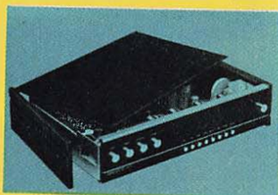
Top, bottom and side panels are removable for total access to circuitry or for custom mounting.
