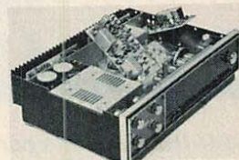
Hinged circuit boards for FM IF, AM IF, Multiplex & Phono Preamp sections.
