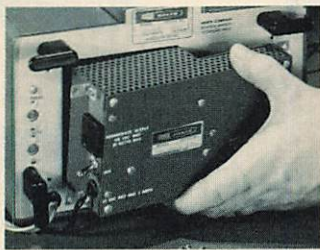
Optional power inverter mounts on rear panel for convenient on-the-road testing capacity.
