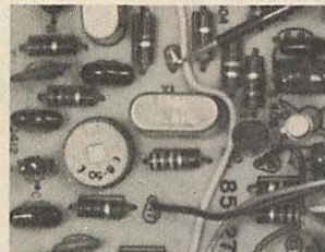
Built-in 500 kHz crystal calibrator for tuning accuracy
