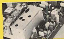
Two ceramic filters contribute to selectivity greater than 60 dB.
