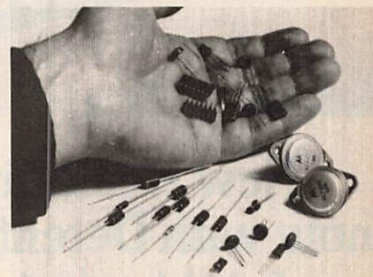
Sophisticated solid-state circuitry includes 23 transistors, 13 diodes and two integrated circuits (ICs).
