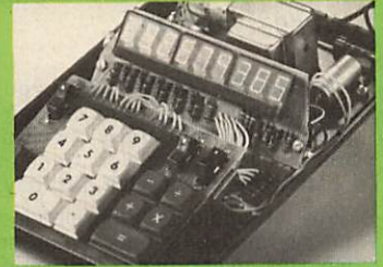
Components mount on one roomy circuit board, and there's an internal adjustment to compensate for high or low line voltage.
