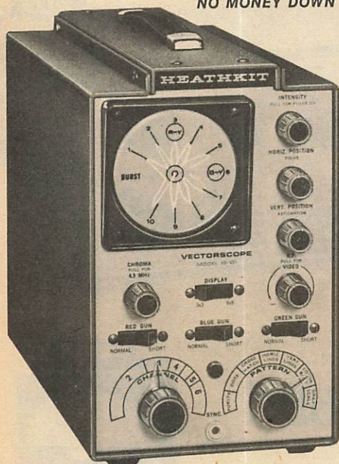
The IO-101 produces 12 patterns plus a clear raster for purity adjustments. All patterns are available at the turn of a knob, either in the familiar 9x9 or the exclusive Heath 3x3 display.
