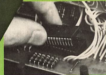
Large scale integrated circuit mounts in socket for easy, trouble-free kitbuilding.
