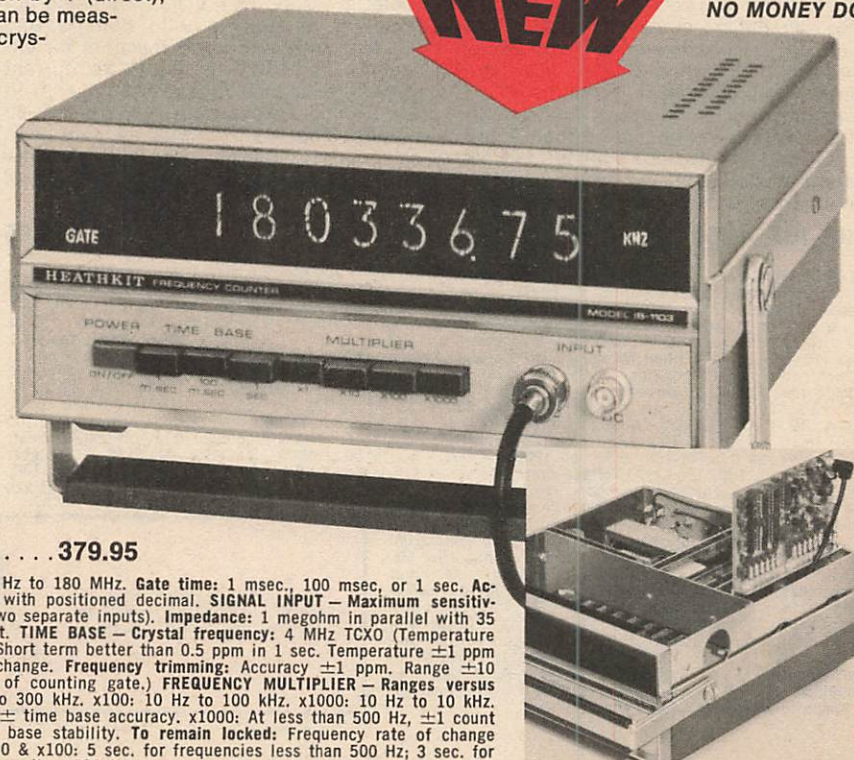
An extender circuit board is provided to allow easy access to the input, time base or frequency multiplier circuit boards for in-circuit servicing.
