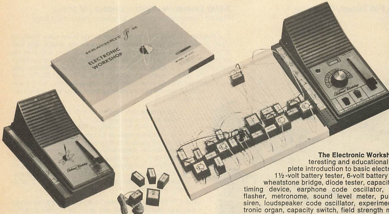
Actual components mount inside modules carrying the component's schematic symbol.
