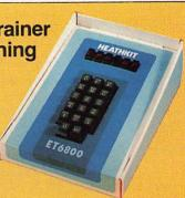
The ET-6800 Microprocessor Trainer functions as a miniature computer with 1K ROM monitor program. Address and data readout on six-digit hexadecimal keyboard gives access to memory locations. Employs an 8-bit parallel NMOS, bus-oriented CPU with 256 bytes of NMOS RAM. Built-in +5 volt DC power supply. Rugged, attractive cardboard cabinet holds the price to an absolute minimum. For 120 VAC, 60 Hz. Measures 3¾" H x 8" W x 10" D.
