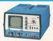
Sweep: Type: Triggered. Range: 200 mS to  $0.2 \mu\text{S}$  in 7 steps, plus variable. Trigger Source: Y1/Y2 External/Line. Trigger Modes: AC/DC/TV/+/-/Slope/Auto/Normal. CRT: 5DEP31F, 8 x 10 cm viewing area, blue-green medium persistence phosphor, 5-inch round flat-face tube. Accelerating Potential: Approximately 1.6 kV. Graticule: Screened. 8 x 10 cm. Power Requirements: 120/240 VAC, 50/60 Hz, 50 watts. Dimensions:  $8^{\prime\prime}\text{Hx}$  13" W x 17" D (20.32 x 33.02 x 48.18 cm).
