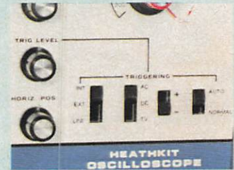
Complete trigger controls include TV coupling for easy triggering on complex TV signals.
