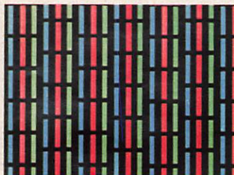
New slot-mask picture tube for greater light output and picture realism.
