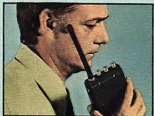
Flexible "rubber duckie" antenna, matched to transceiver is included, plus jack for external antenna.
