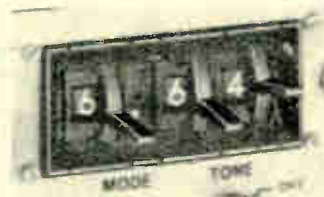
Front Panel Lever Switches Select Any Frequency in Any 4 MHz Segment of the HW-2036A's 143.5 to 148.5 MHz Operating Range.
