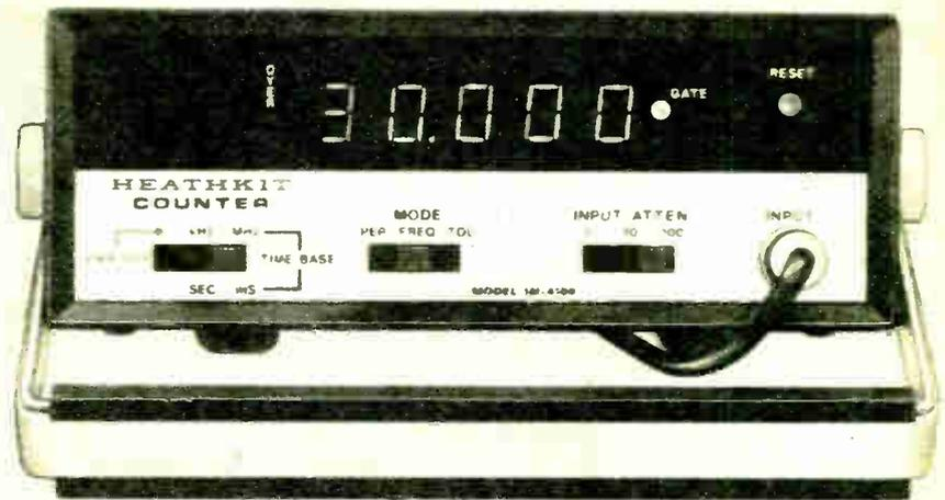
**The Heathkit IM-4100 is a frequency counter and much more – Counts frequency to 30 MHz, period to 99.999 seconds, events to 99,999**
