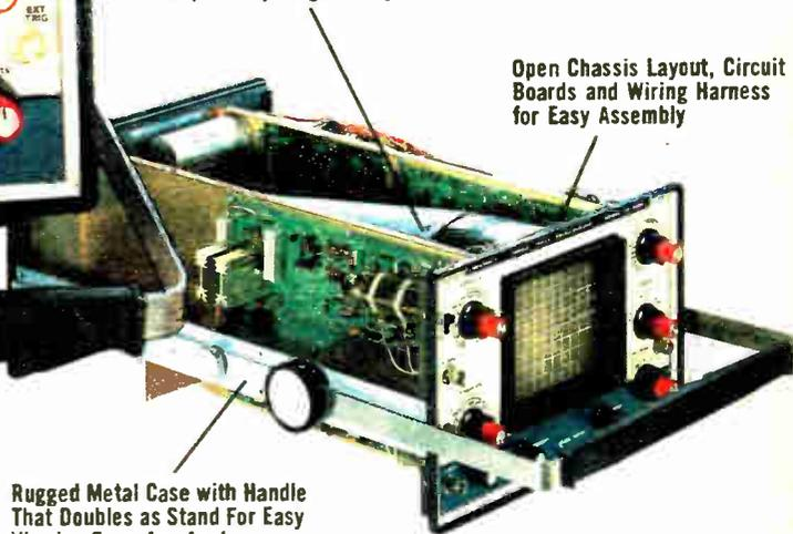
Rugged Metal Case with Handle That Doubles as Stand For Easy Viewing From Any Angle
