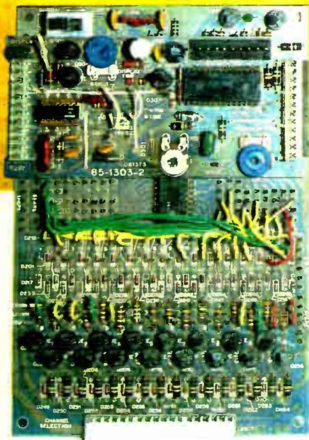
The "heart" of the GR-2000 is the channel selector circuit board. It provides the direct electronic tuning, the dot generator for color alignment, and positions and controls the numerical channel display.
