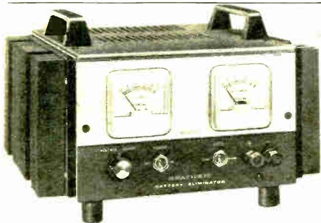
**IP-2715 SPECIFICATIONS:** Output Voltage: variable from 9-15 VDC. Output Current: 12 amps continuous, 20 amps intermittent (per derating curve in manual). Ripple: less than 1% at full load. Regulation: less than 2% variation from no load to full load. Fuses: 7A, 3 AG slow-blow primary; 20A, 3 AG output. **Power Requirement:** 110-130 VAC, 7A or 220-260 VAC, 3.5 A, 60/50 Hz. **Dimensions:** 5 1/4" H x 11" W x 11" D.
