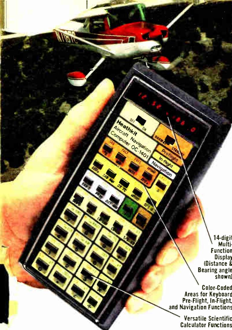
14-digit Multi-Function Display (Distance & Bearing angle shown)
