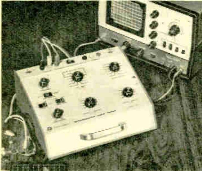
The fast, easy way to check semiconductor parameters is with your oscilloscope and the IT-3121 Curve Tracer
