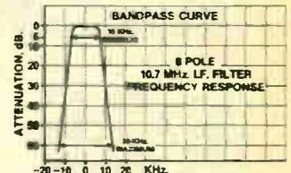
An 8-pole IF Crystal Filter greatly reduces adjacent channel interference for clear, static-free transmission and reception.
