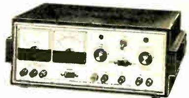
IP-2717 SPECIFICATIONS: Additional Outputs: 0 to -100 VDC at 1 mA variable bias voltage, 6.3 VAC at 4 amps., 12.6 VAC at 2 amps. (25 VA max. AC load), filament voltage. Regulation: Output variation less than 1% from no load to full load. Ripple: Less than 10 millivolts rms. Output Impedance: Less than 10 ohms, DC to 1 MHz. Meters: Voltmeter 0-400 V or 0-150 V; Milliammeter 0-150 mA. Power Requirement: 120/240 VAC, 60/50 Hz, 150 W max. Dimensions: 5 1/8" H x 13 3/4" W x 11" D.
