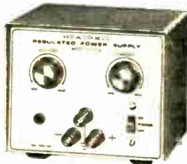
IP-2728 SPECIFICATIONS: Ripple and Noise: Less than 5 mV. Current Output: 500 mA maximum continuous load. Current Limiting: Adjustable from 10 mA to over 500 mA. Transient Response: 25 microseconds. Output Impedance: 0.5 ohm or less to 100 kHz. Power Requirement: 120/240 VAC, 60/50 Hz, 15 W at full load. Dimensions: 4 3/8" H x 5 1/2" W x 5 3/4" D. Programming: AC or DC, 5000 ohm input resistance.
