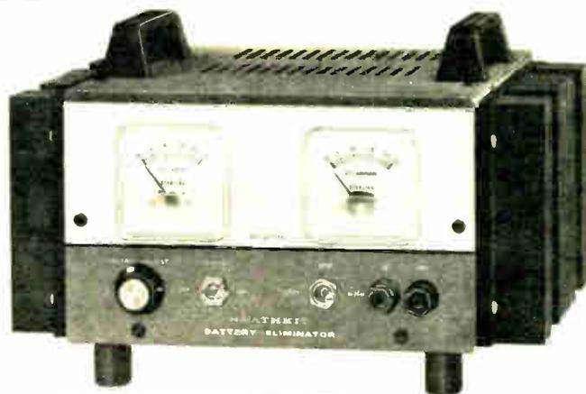
IP-2715 SPECIFICATIONS: Output Voltage: variable from 9-15 VDC. Output Current: 12 amps continuous, 20 amps intermittent (per derating curve in manual). Ripple: less than 1% at full load. Regulation: less than 2% variation from no load to full load. Fuses: 7A, 3 AG slow-blow primary; 20A, 3 AG output. Power Requirements: 110-130 VAC, 7A or 220-260 VAC, 3.5 A, 60/50 Hz. Dimensions: 5 1/4" H x 11" W x 11" D.
