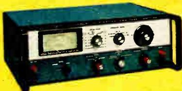
**Harmonic Distortion Analyzer.** The Heathkit IM-5258 Harmonic Distortion Analyzer is a professional-grade total harmonic distortion (THD) analyzer. Its outstanding sensitivity and bandwidth let you measure total harmonic distortion at levels as low as 0.03 percent, from 5 Hz to 100 kHz, with 5 percent full scale accuracy. Not for use in strong RF fields. For 120/240 VAC, 50/60 Hz. Dimensions, 5 5/8" H x 15" W x 11 1/2" D.
