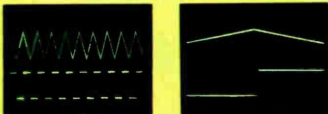
The delayed sweep takes the user selected portion of the waveform (intensified portion in the left picture) and magnifies it the desired number of times for closer examination (right picture).
