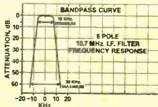
The HW-2036A's 8-pole IF crystal filter greatly reduces adjacent channel interference — an important feature as 2-meters grows in popularity and the band becomes more crowded — to give you clear, static-free FM transmission and reception.
