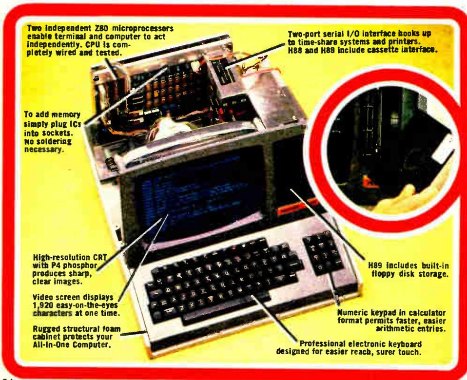
Two independent Z80 microprocessors enable terminal and computer to act independently. CPU is completely wired and tested.
