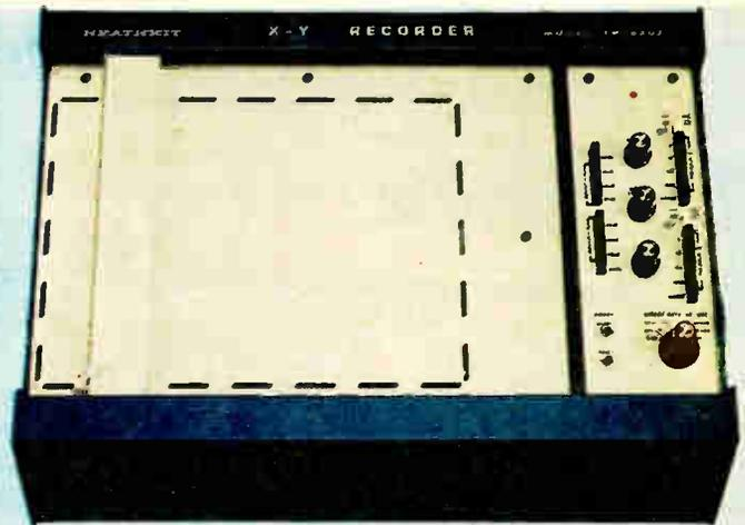
The easy-to-use IR-5207 Chart Recorder is precise enough for your most demanding measurements. Precise to  $\pm 0.5$  percent of full scale (dead band and non-linearity error is less than 0.25 percent of full scale.)
