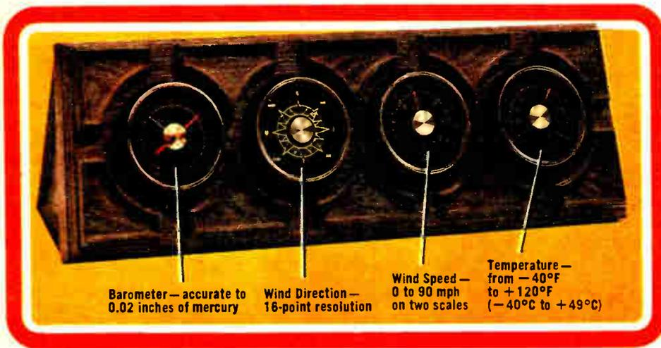
Barometer — accurate to 0.02 inches of mercury
