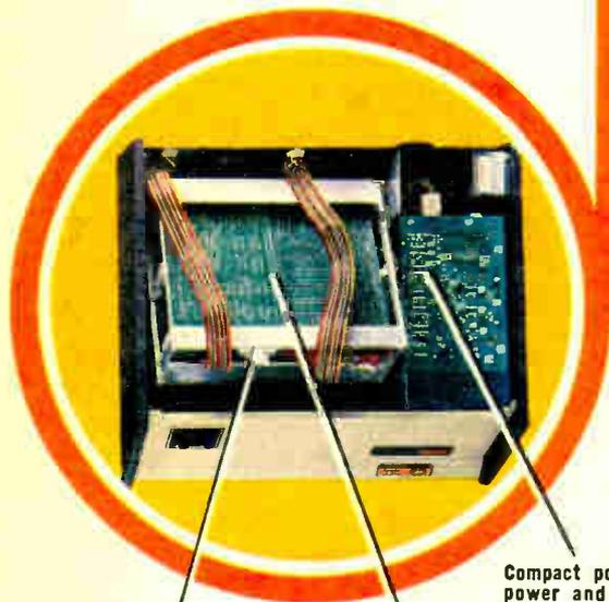
Rugged steel chassis and extra-thick backplane with heavy, solid connectors for added strength and years of reliable performance.
