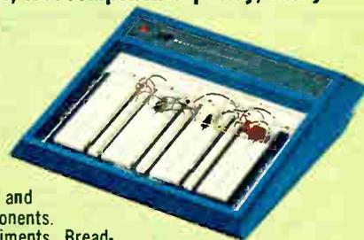
The Heathkit Circuit Breadboard is a great convenience tool. Design and test circuits. Test components. Perform your own experiments. Breadboard features solderless sockets for fast, easy connections and tear-downs. Plus reliable built-in power supply.
