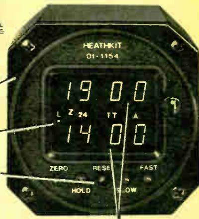
4-digit red LED displays with automatic dimming.
