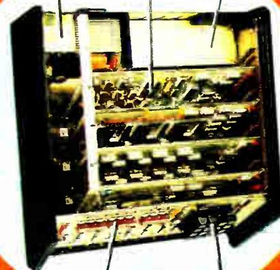
8080A-based, with front panel keyboard, digital readout and 7 plug-in board positions
