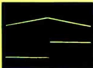
The delayed sweep takes the user selected portion of the waveform (intensified portion in the left picture) and magnifies it the desired number of times for closer examination (right picture).
