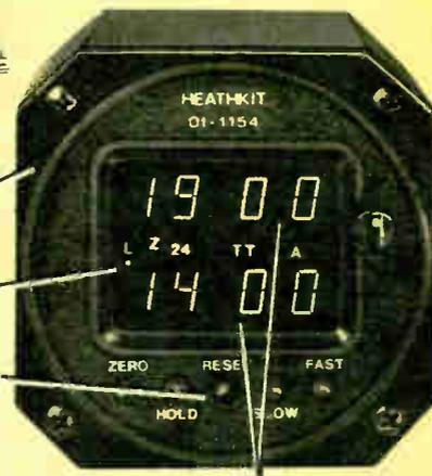
4-digit red LED displays with automatic dimming.
