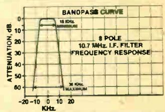
An 8-pole IF crystal filter greatly reduces adjacent channel interference for clear, static-free FM transmission and reception.
