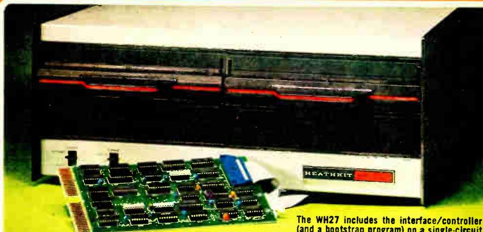
The WH27 includes the interface/controller (and a bootstrap program) on a single-circuit card at no extra charge.
