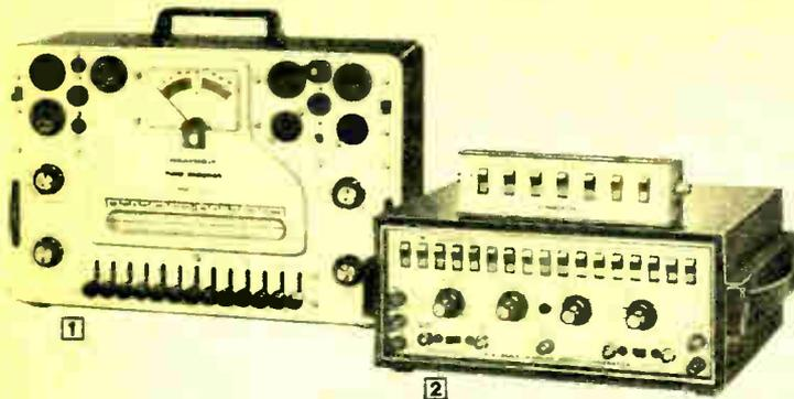
**1 Low-Cost Heathkit Tube Checker.** Essential for radio-TV servicing! Tests tubes on the basis of total emission, for shorts, leakage, open elements, and filament continuity. Has good-?bad indicator to show relative quality, neon bulb indicator for filament continuity and leakage or shorts between elements. Easy-to-operate roll chart.
