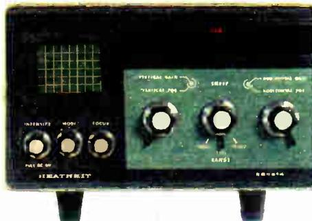
Monitors transmitted SSB, CW, & AM signals up to 1 kW from 80-6 meters. Shows nonlinearity, insufficient or excessive drive, poor carrier or sideband suppression, regeneration, parasitics and key clicks. Manual includes 40 CRT displays including: 21-transmit envelope patterns, 7-trapezoid patterns, 6-RTTY cross patterns (for proper shift, mark and space adjustment), and 6-CW patterns. Solid-state.
