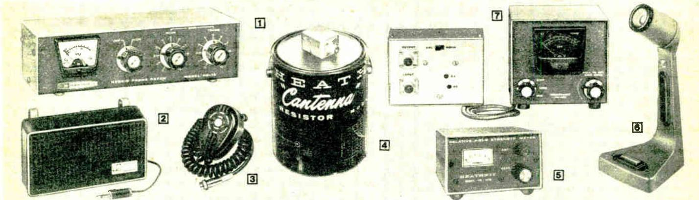
**1** Heathkit Hybrid Phone Patch. Add the versatility of phone patch capability to your shack with Heath's HD-15. Individual receiver/transmitter line gain controls simplify adjustment and the HD-15's VU meter continuously monitors the unit's output. Interfacing with your system is a simple matter. Matches 3-16 ohm speakers and hi-Z or 600 ohm inputs. PTT operation. 2 $\frac{1}{2}$ " H x 9 $\frac{1}{4}$ " W x 3 $\frac{3}{8}$ " D. Kit HD-15, Shpg. wt. 3 lbs. .... 37.95
