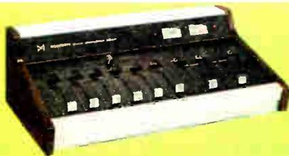
**TM-1626 SPECIFICATIONS:** Frequency Response: 40-20,000 Hz,  $\pm$ 1 dB. Distortion: 0.5% maximum at outputs from 50 mV to 6.5 volts. Output Impedance: 150 ohms. Power Requirement: 120/240 VAC, 60/50 Hz, 15 watts maximum. Dimensions: 5½" H x 16" W x 9½" D.
