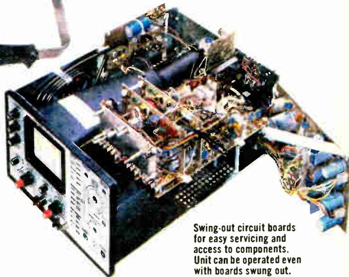
Swing-out circuit boards for easy servicing and access to components. Unit can be operated even with boards swung out.
