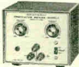
Continuously adjustable from 1-15 VDC at 500 mA output. Has 500 mV line and load regulation and fully adjustable current limiting. AC or DC programming capability lets you control output voltage from another source.
