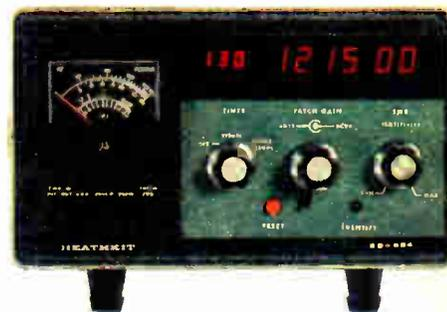
Features 24-hour digital clock; ten-minute ID timer; RF wattmeter with 200 or 2000 watt full scale ranges; SWR bridge with sensitivity control; phone patch that can be used manually or with VOX control. Wattmeter impedance is a nominal 50 ohms. The phone patch provides at least 30 dB isolation. Input impedance is 600  $\Omega$ . Matches 3-16  $\Omega$  receiver outputs, and 600  $\Omega$  or hi-Z transmitter input.
