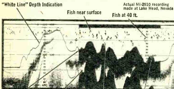
Bottom Depth      Second Echo of bottom      Fish near bottom      Normal Depth Indication
