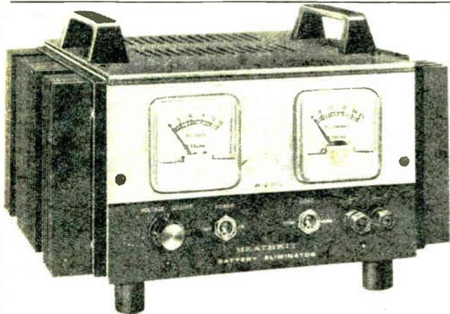
**IP-2715 SPECIFICATIONS:** Output Voltage: variable from 9-15 VDC. Output Current: 12 amps continuous, 20 amps intermittent (per derating curve in manual). Ripple: less than 1% at full load. Regulation: less than 2% variation from no load to full load. Fuses: 7A, 3 AG slow-blow primary; 20A, 3 AG output. Power Requirement: 110-130 VAC, 7A or 220-260 VAC, 3.5 A, 60/50 Hz. Dimensions: 5¼" H x 11" W x 11" D.
