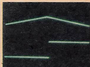
The delayed sweep takes the user-selected portion of the desired waveform (intensified portion in left photo) and magnifies it the desired number of times, to allow for closer examination (as seen in photo at right).
