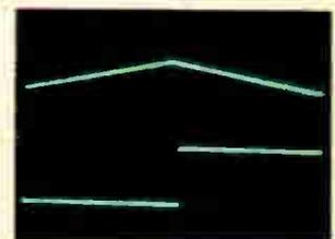
The delayed sweep takes the user-selected portion of the desired waveform (intensified portion in left photo) and magnifies it the desired number of times, to allow for closer examination (as seen in photo at right).
