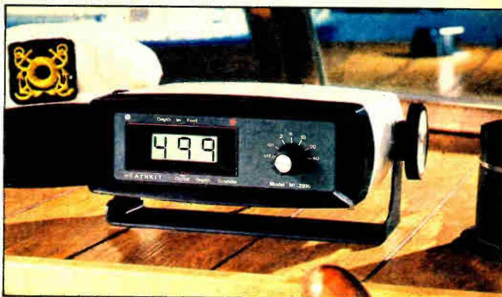
**MI-2916 SPECIFICATIONS:** Depth Ranges: 2.0' to 9.9' and 10' to 499'. Autoranging. Display: LCO with auto night light. Frequency: 200 kHz. Accuracy: ± 5% +1 count. External Control: Off-On switch. Alarm Settings: 2', 4', 10', 20', 40'. Internal Controls: Keel offset, 0' to 7'. Operating Temperature Range: 32°F to 122°F (0° to 50°C). Power Requirement: 10 to 17.7 VDC. Average Current: 25 mA. (110 mA with night light). Alarm: Audible and Visual.
