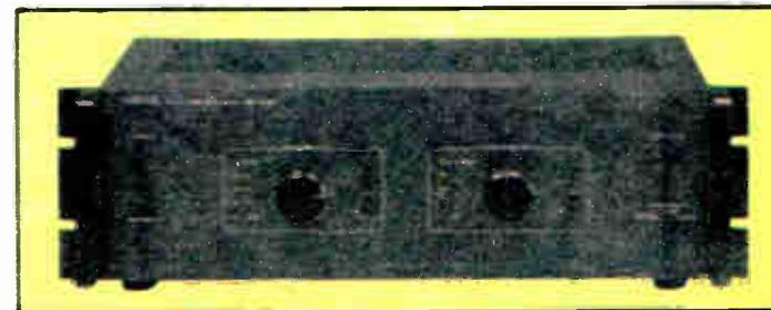
**SPECS:** Expansion: -4 dB to +4 dB. Freq. Resp.: 20 Hz to 20 kHz. THD: < .01%. Hum & Noise: -70 dB. High Filter: -3 dB, 7 kHz, 12 dB/octave. Input Overload: 5 VRMs min. at 1 kHz. Power Req.: 120/240 VAC, 50/60 Hz. Dim.: 5.75" H x 19" W x 14" D.
