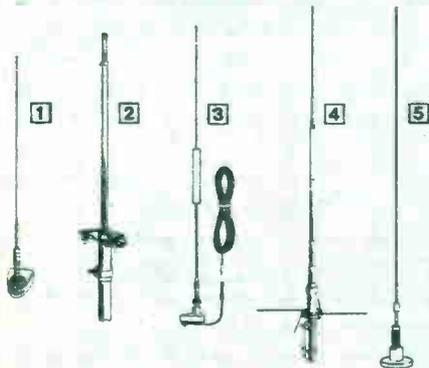
1 Hustler Standard Gain 2M Mobile Antenna. 3/8 wavelength rear deck whip. 3.4 dB gain, 1.1:1 SWR. Handles 100 watts. 47" radiator. 17" coax, connectors included. Antenna removable from mount.
